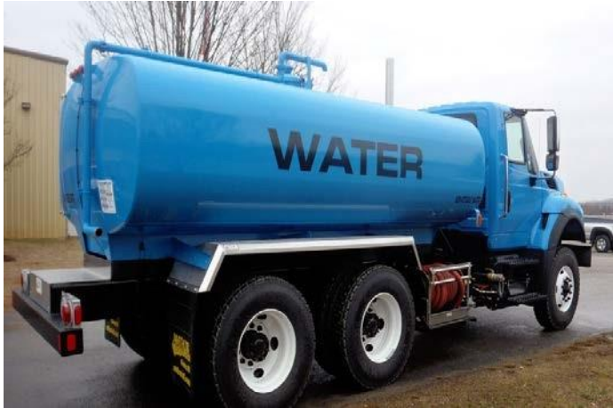
Image 4: Water tank truck to supply water to the site
