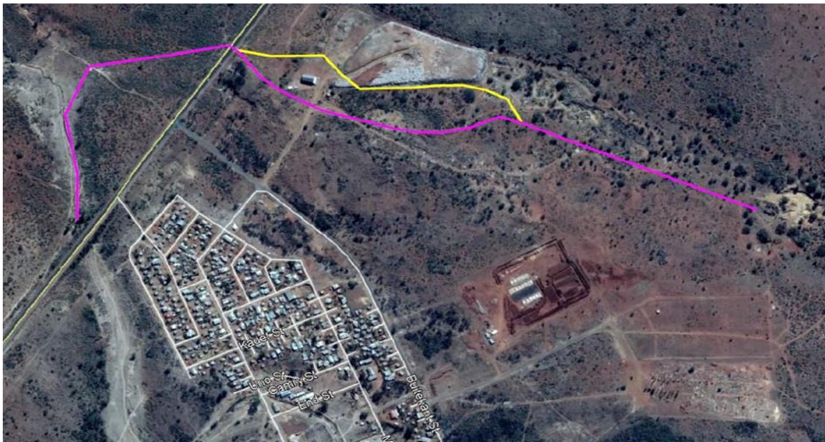
Figure 2: Proposed Bulk Sewer Pipelines Layout.
