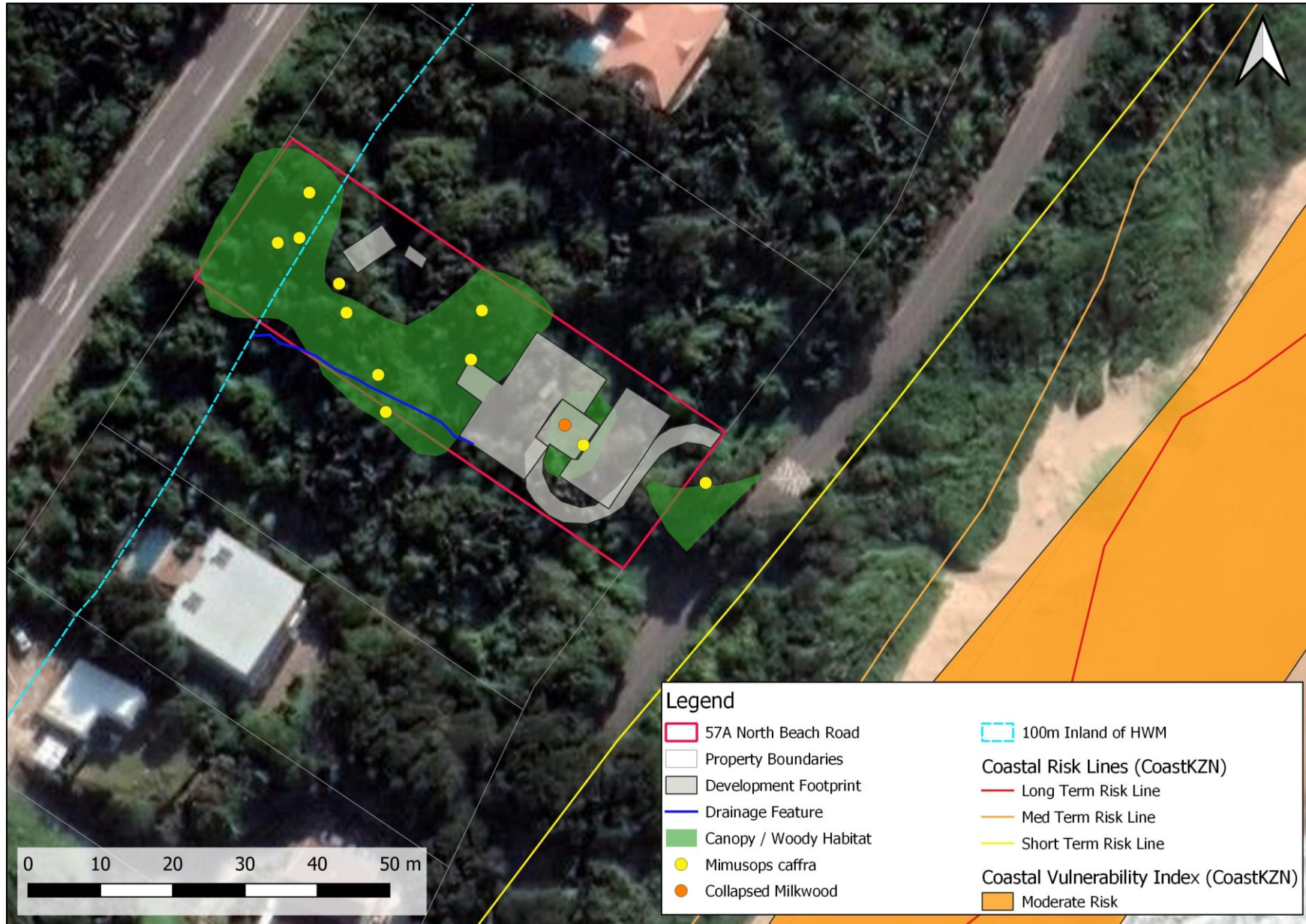
Figure 3: Map Superimposing the Proposed Activity and Associated Infrastructure on the Environmentally Sensitivities of the Site.
