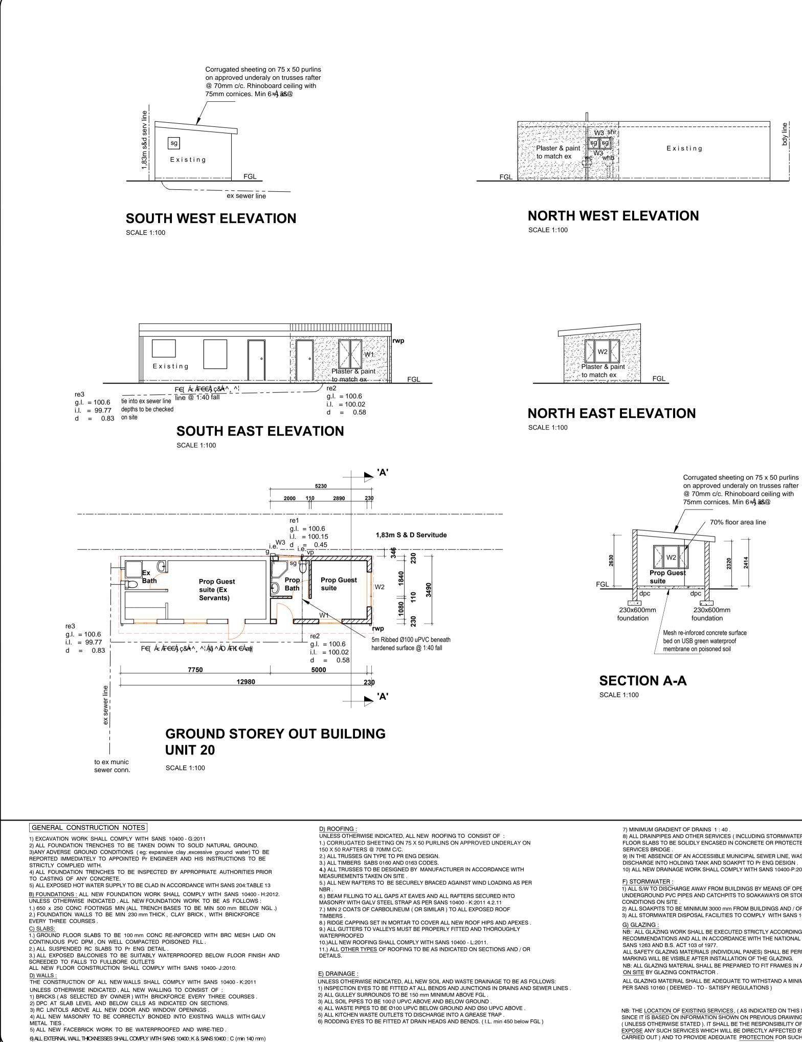
7) ALL LOAD BEARING WALL THICKNESSES TO BE MIN 190 mm.
