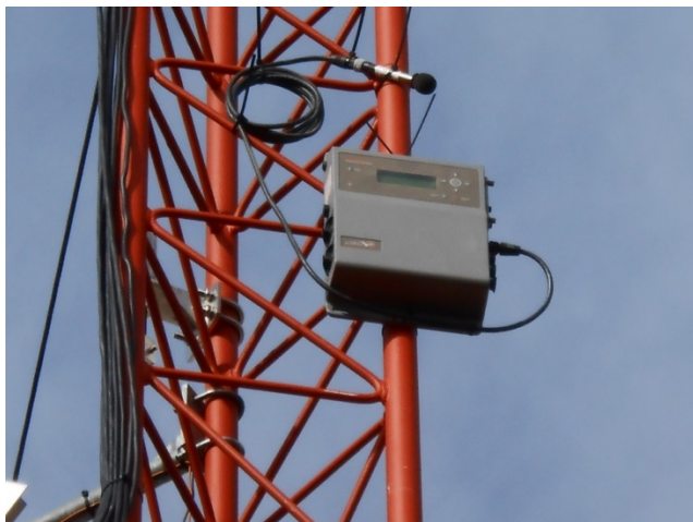
Figure 1. SM3 bat detector unit and microphone installed on a met mast at a height of 10 m above the ground.
