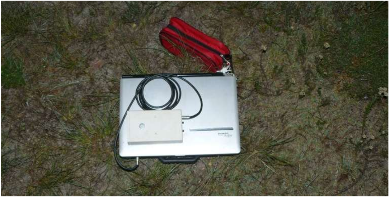
Figure 7: A Time expansion type bat detector connected to a laptop
