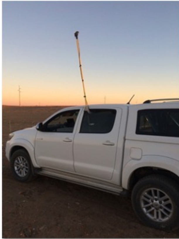
Figure 3: Microphone mounted on a vehicle for transects
