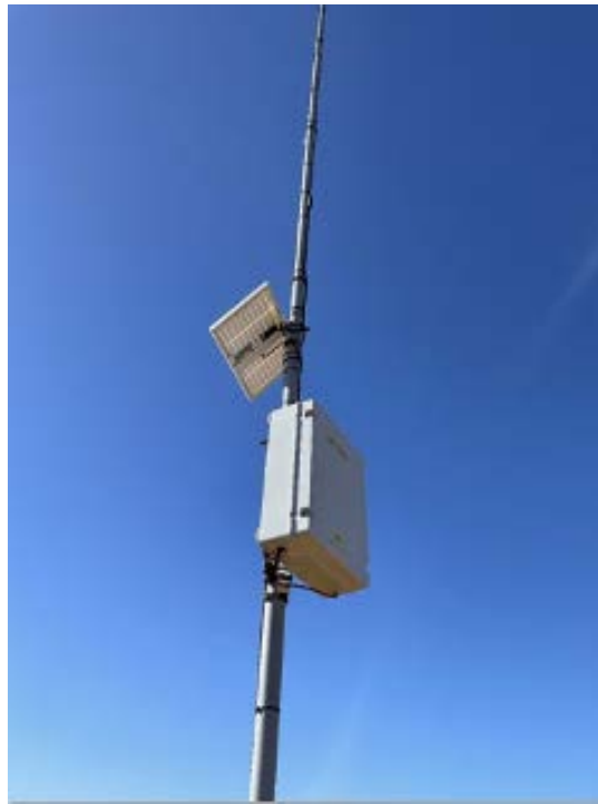
Figure 2: Monitoring Station I, the 10 m Mast on the proposed wind farm site
