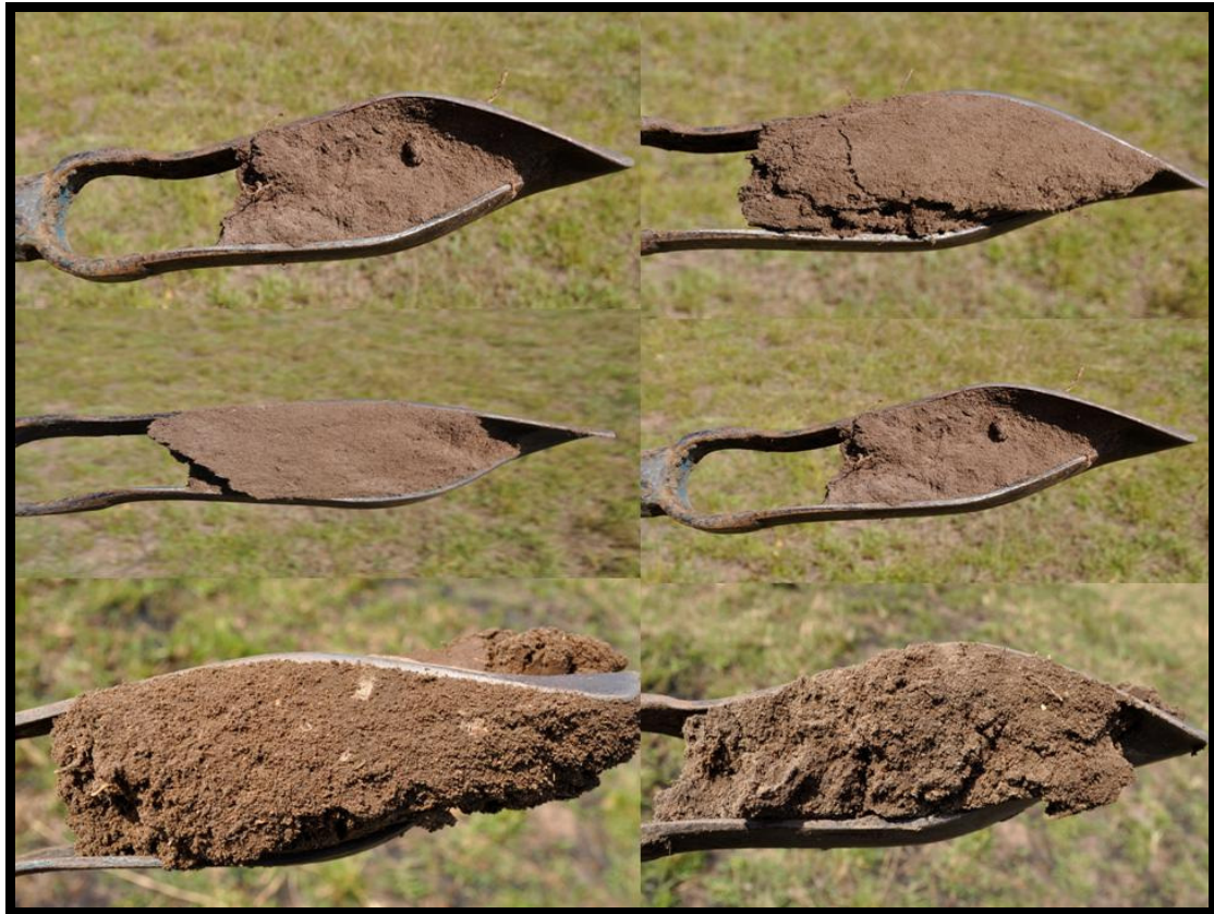
Figure10. A collage of photographs displaying soil auger samples. The majority of the site comprises well drained brown sandy to sandy clay-loams. No hydric indicators were observed within the majority of soils augers taken from the hillslopes and footslopes. Hydric indicators were observed adjacent to the perennial and non-perennial drainage lines as well as within the flood bench of the Tugela River.
