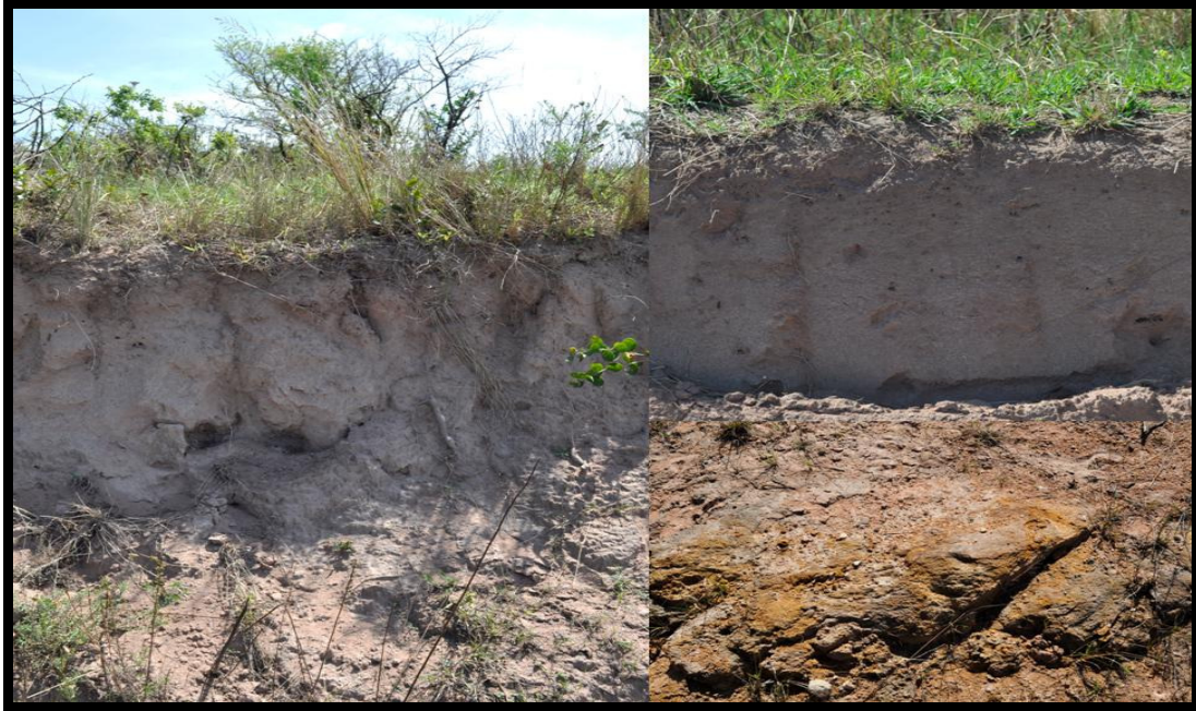
Figure6. The geology of the site is dominated by Ordovician Natal Group sandstone. The depth of the soils varied throughout the site. Relatively deep soils (1.2 m) occur within certain areas whilst other areas are situated on a very shallow soil layer (< 50cm). The sandstone layer is evident within eroded areas as well as regularly scraped access roads.
