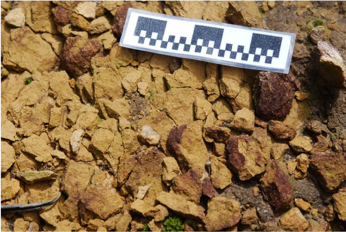
Plate 9-2: Crumbly yellow weathered diamictite exposed in a prospecting pit in the extreme east of the study area (Figure 9-1, point 1).
