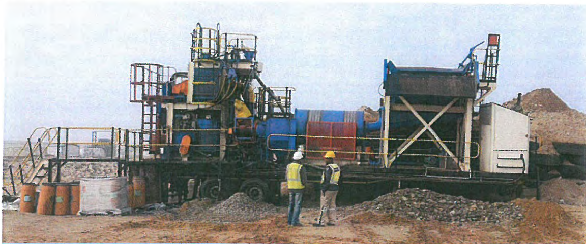
Annexure 2: Figure 2 - New WCR 10tph mobile DMS Prospecting Plant in transit (top) and in operation (bottom)
