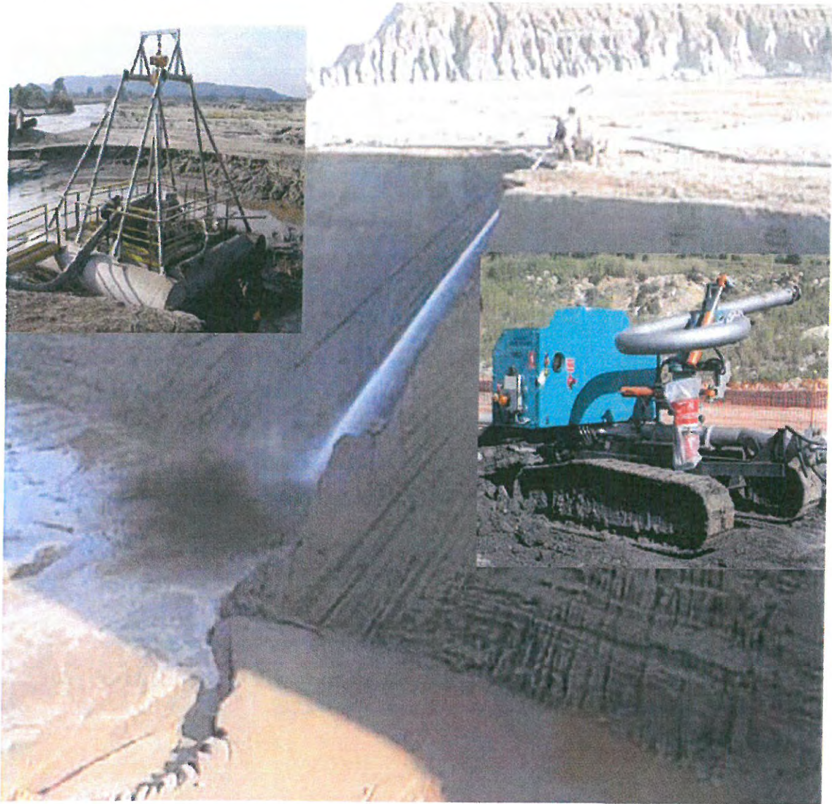
Annexure 1: Figure 3- Diagram illustrating the hydraulic mining method (top) and discharge of slurry to sea for beach accretion and seawall mining (middle and bottom).
