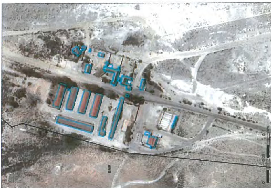
Figure Q-B : Plan from NGI Imagery with shapefile blue outlines of buildings, giving building footprint area in m 2 in shapefile tables
