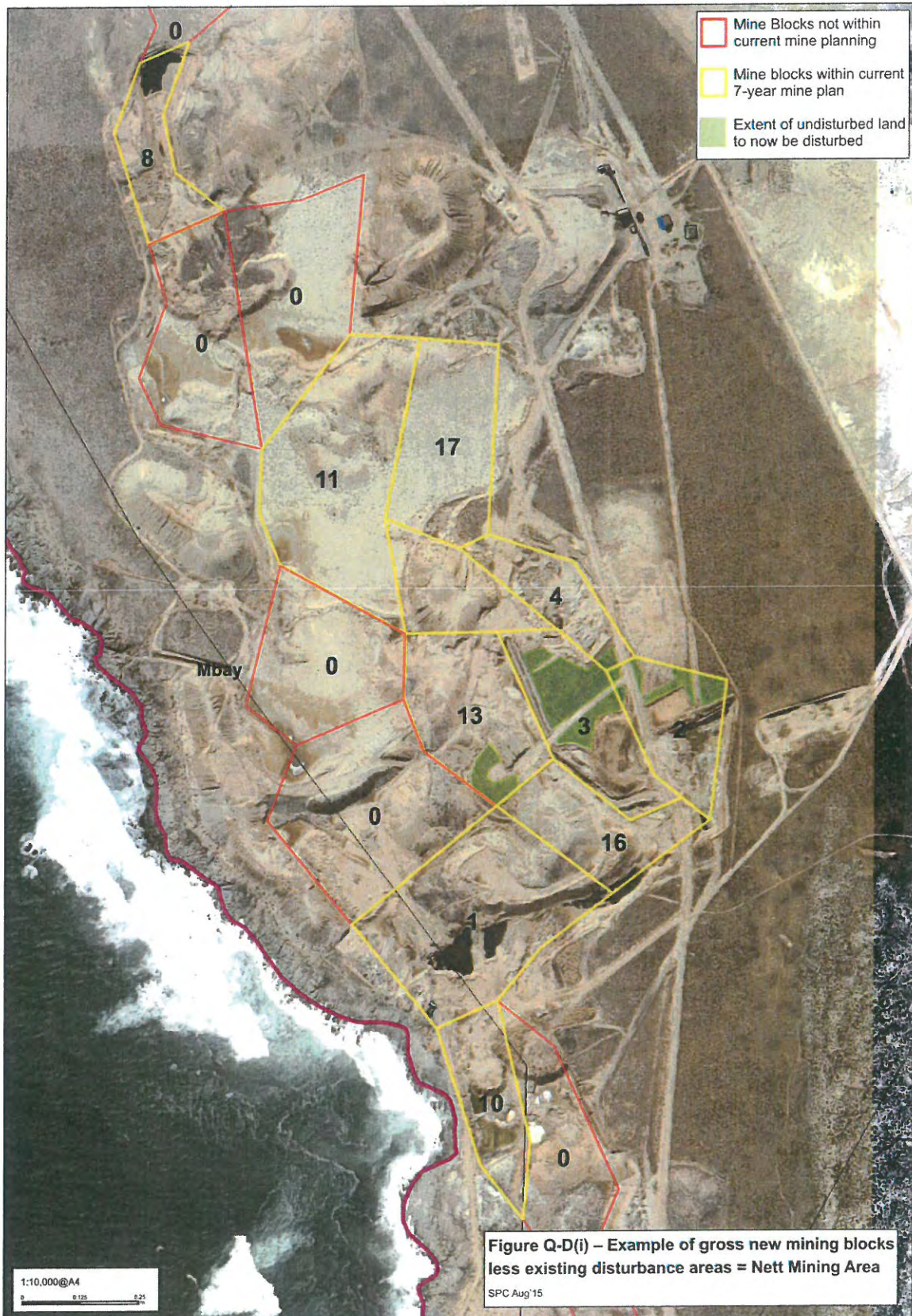
Figure Q-D – Example of gross new mining blocks (yellow) less existing disturbance areas = Nett Mining Area (virgin area to be disturbed (green))
