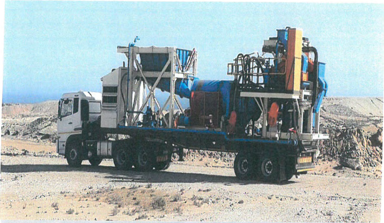
Appendix 4.6: New 10tph mobile Dense Media Separator (DMS) prospecting plant
