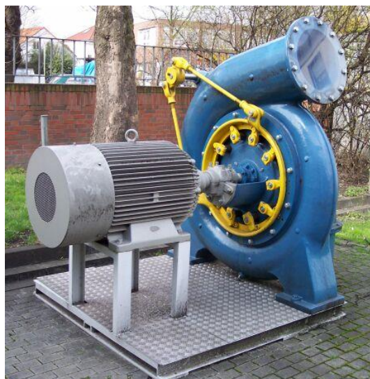
Figure 20 | Francis Turbine and generator. [source: [source: http://en.wikipedia.org , 5 July 2013]]
