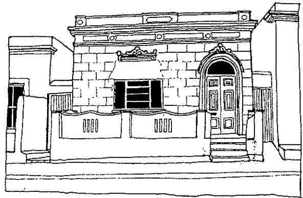
Fig 20. The plaster surround is damaged and the facade spoilt when a sash window is replaced with a horizontal casement.
