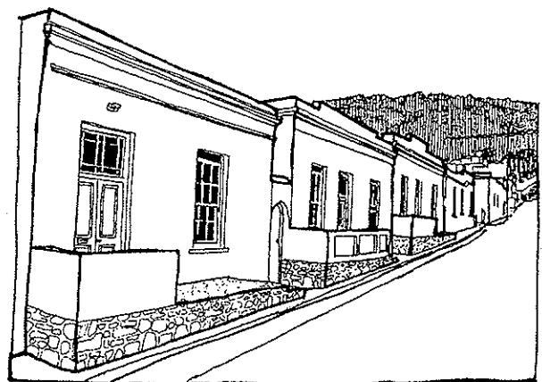
Fig 39. The repetition of narrow facades with elements such as cornices, tall openings and stoeps establishes a regular rhythm in the streetscape.
