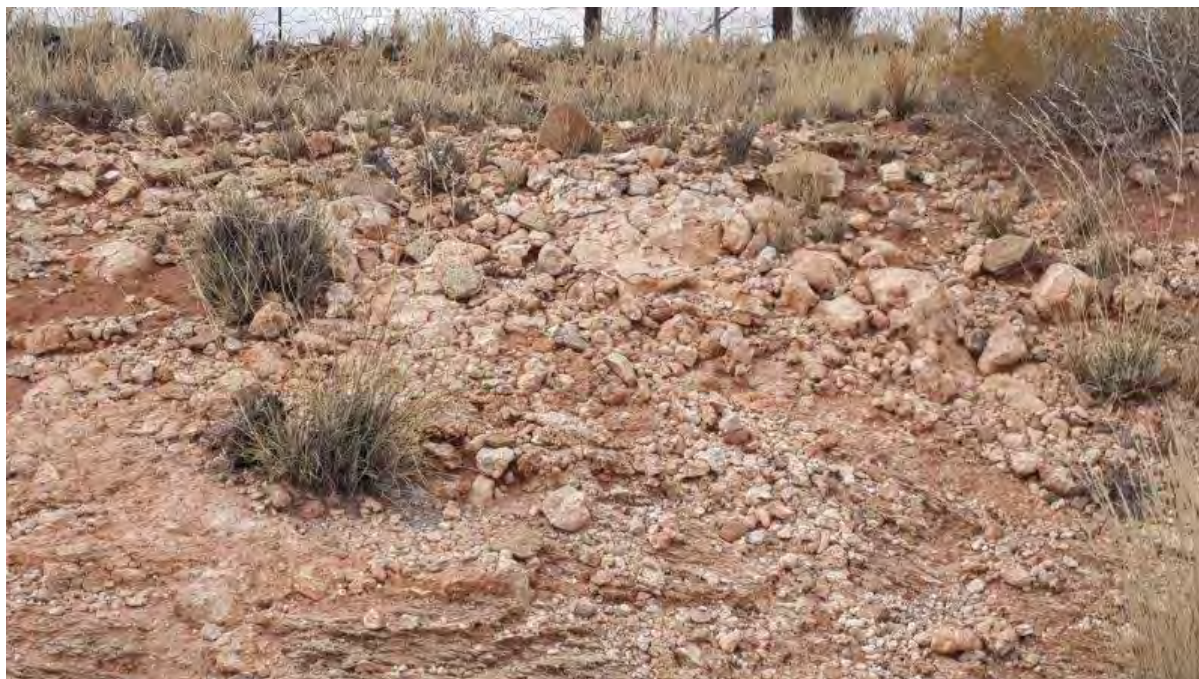
Figure 11.5: Photograph from the area of typical soil profile on the side of an excavation showing shallow hard-pan carbonate horizon (Coega soil form).
