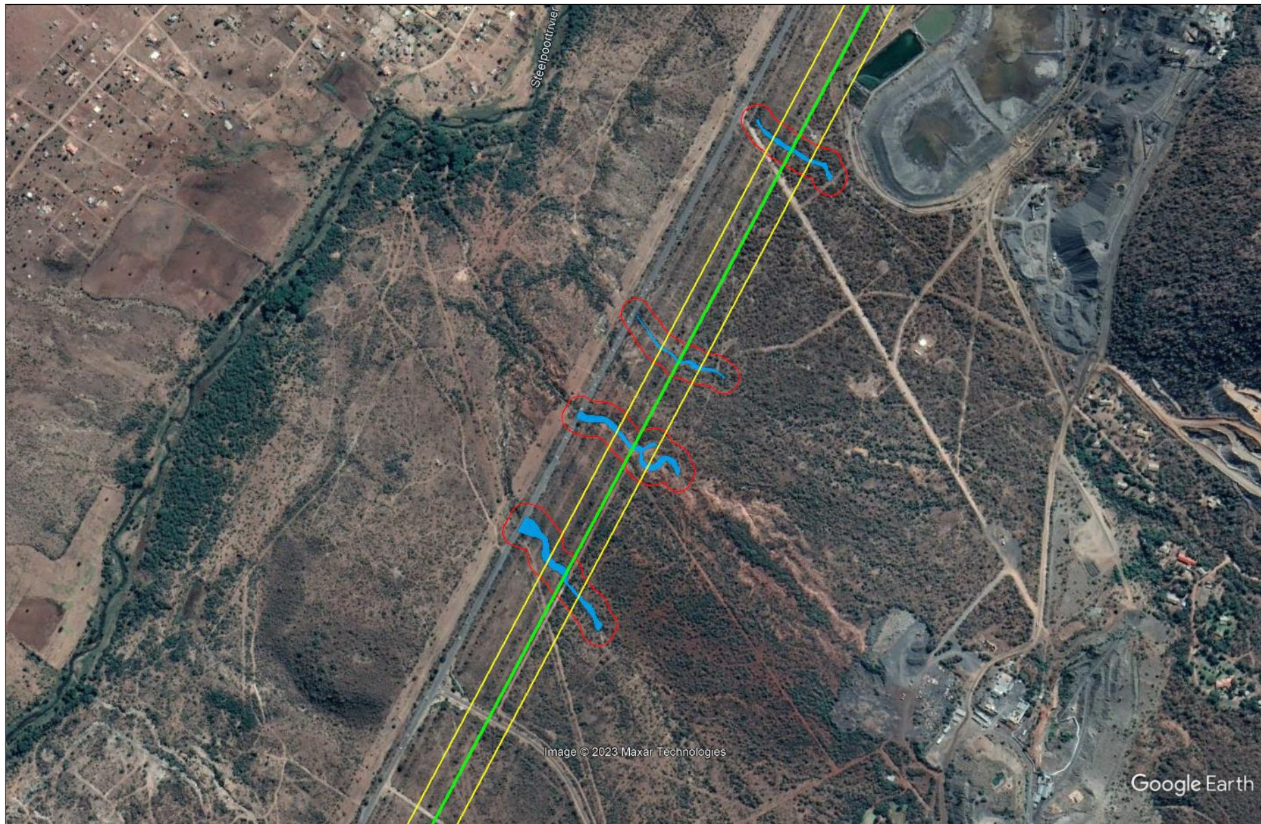
Figure 11. Watercourses and associated 32m buffer zones (Blue=Tributaries; Red=32m buffer zones; Yellow=100 m corridor; Green=Proposed Deviation) (Source: Google earth 2023).
