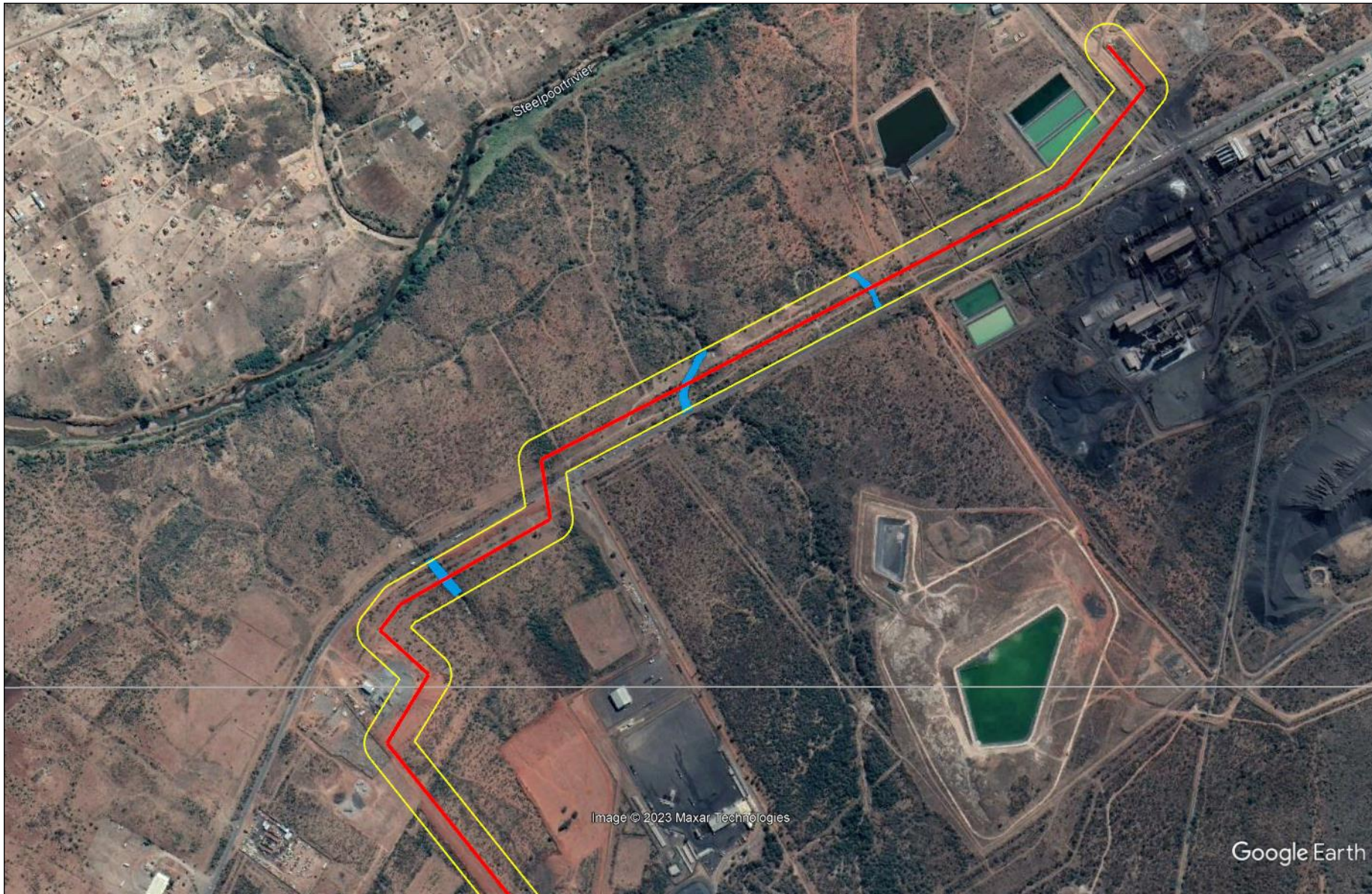
Figure 3. Watercourses identified in the study area (Yellow=100 m corridor; Red=Proposed deviation route; Light blue=Tributaries) (Source: Google Earth, 2023)
