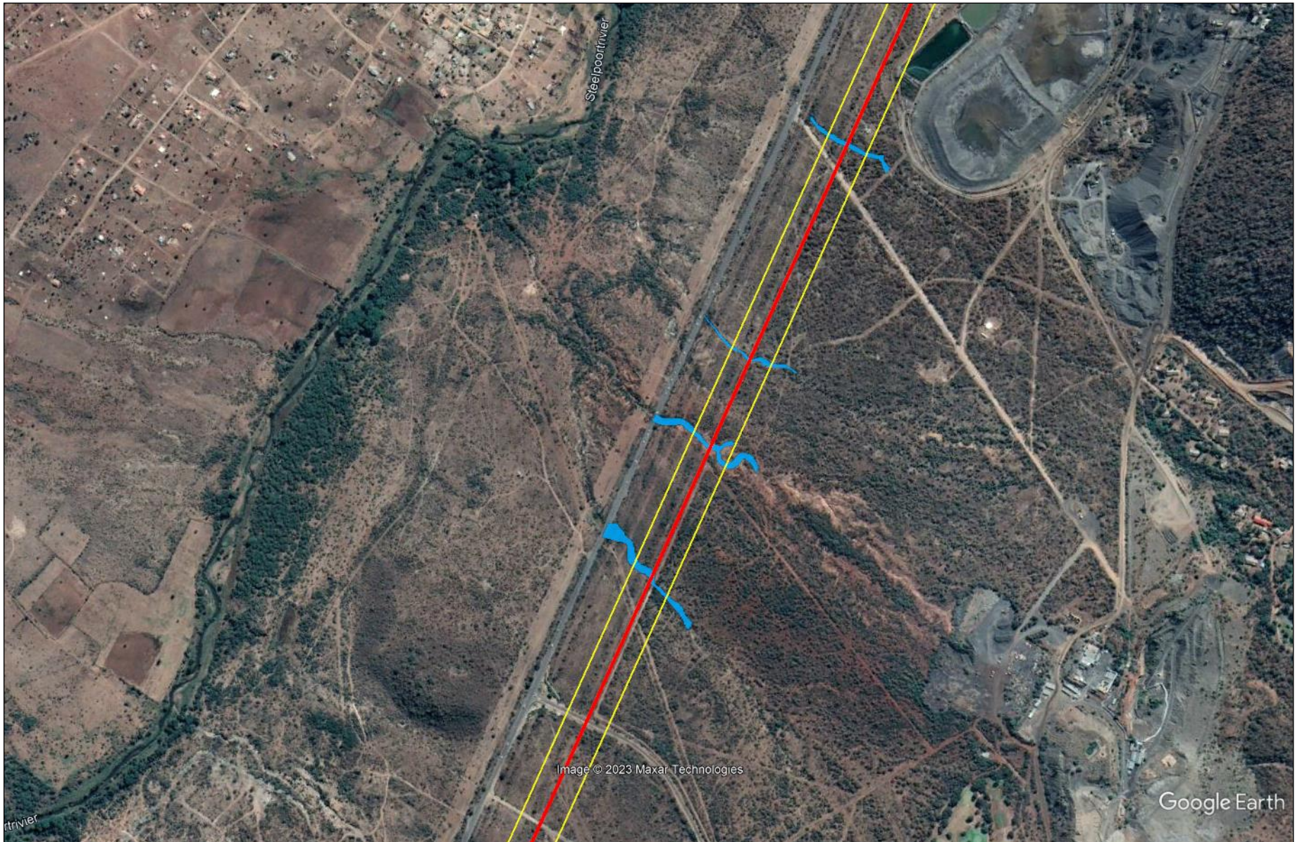
Figure 5. Watercourses identified in the study area (Yellow=100 m corridor; Red=Proposed deviation route; Light blue=Tributaries) (Source: Google Earth, 2023)
