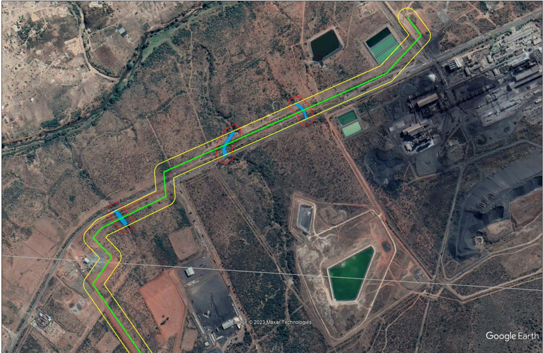
Figure 9. Watercourses and associated 32m buffer zones (Blue=Tributaries; Red=32m buffer zones; Yellow=100 m corridor; Green=Proposed Deviation) (Source: Google earth 2023).
