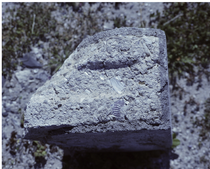
Fig 8. A sample of limestone brick found on Robben Island. A typical example of the quality of brick produced. It appears if the mortar contains cement, which should be analysed to determine the mortar mix for the restoration work.
