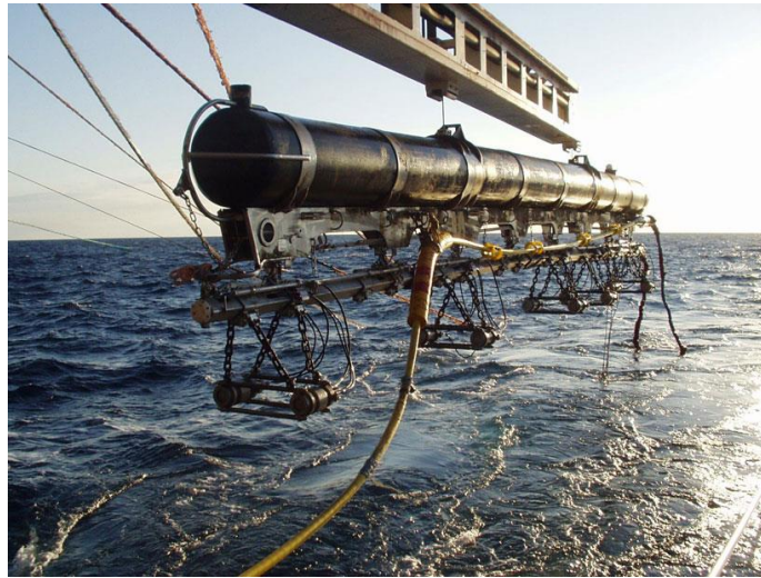
Figure 6-4: A typical seismic source / airgun array
