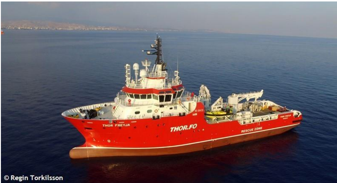
Figure 6-13: Example of a typical seismic escort vessel (M/V Thor Freyja)
