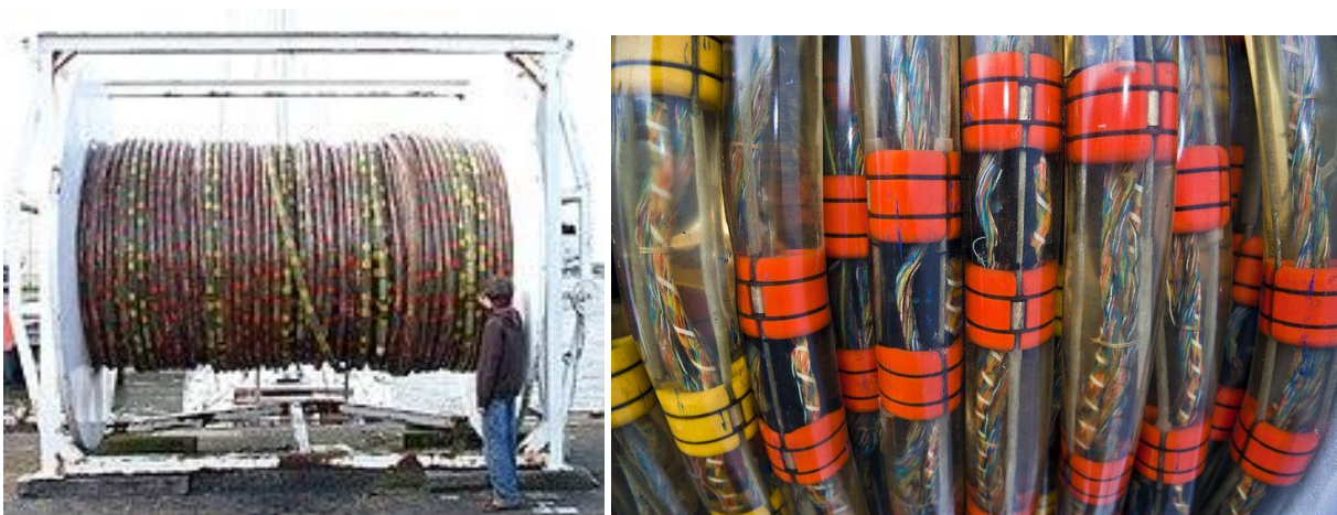
Figure 6-8: Example of a hydrophone streamer
