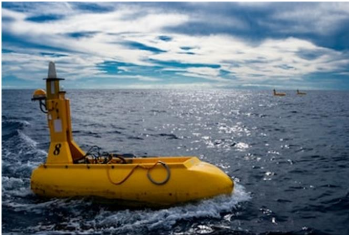
Figure 6-9: Example of a tail buoy
