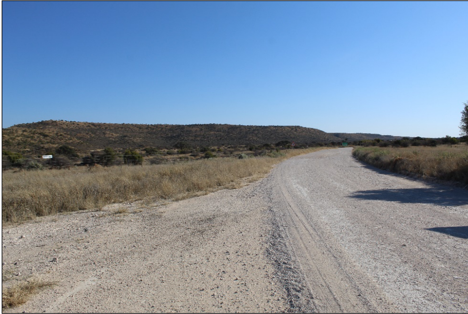
Figure 4: The line will follow the south side of the road servitude (right side of the road in this picture). The road exposes the calcrete horizon.
