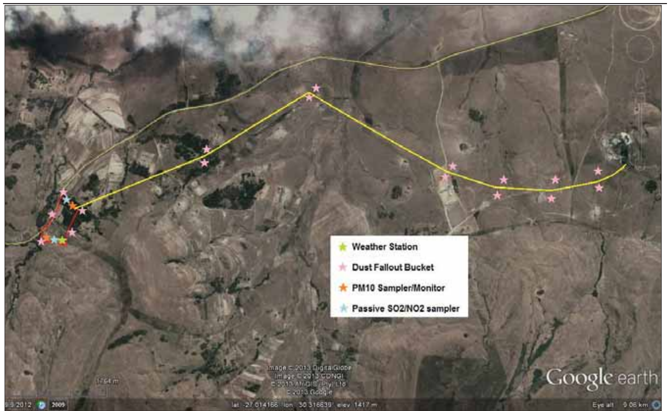
Figure 14.4 Indicative Air Quality Monitoring Locations
