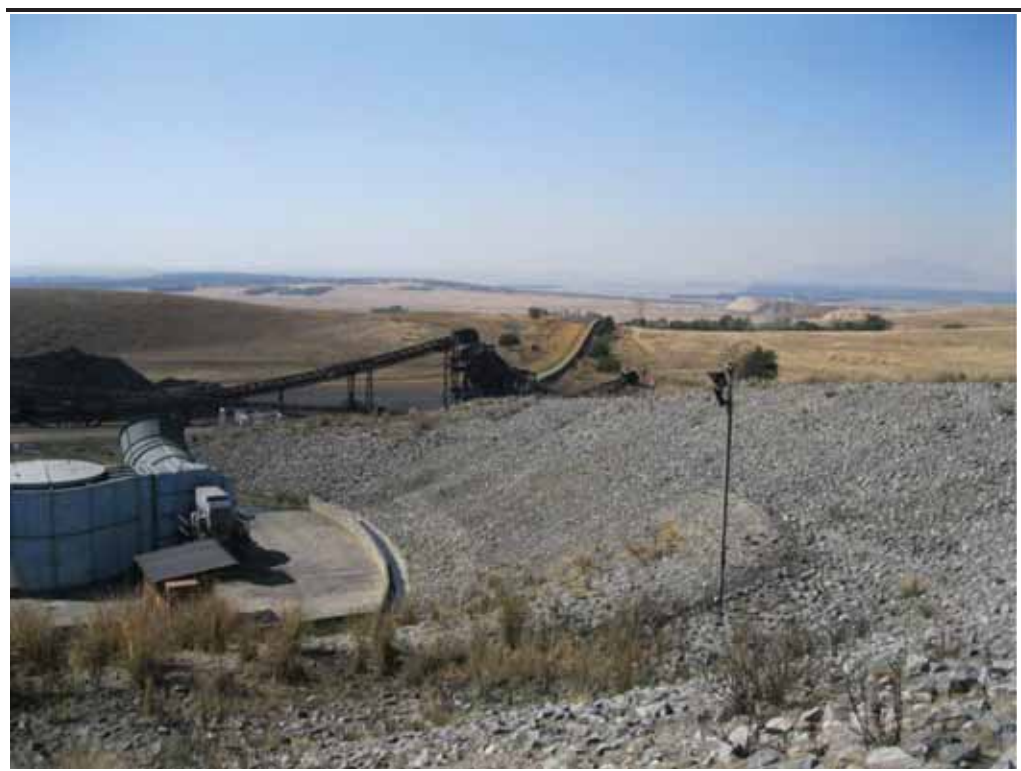
Figure 3.8 Typical Conveyor Belt System in the Background Transporting Coal to a Wash Plant
