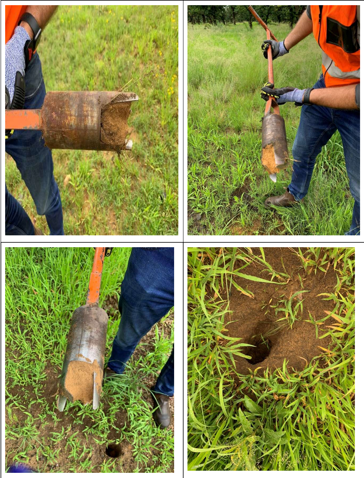
Figure 8-4: Augered Soils on Site
