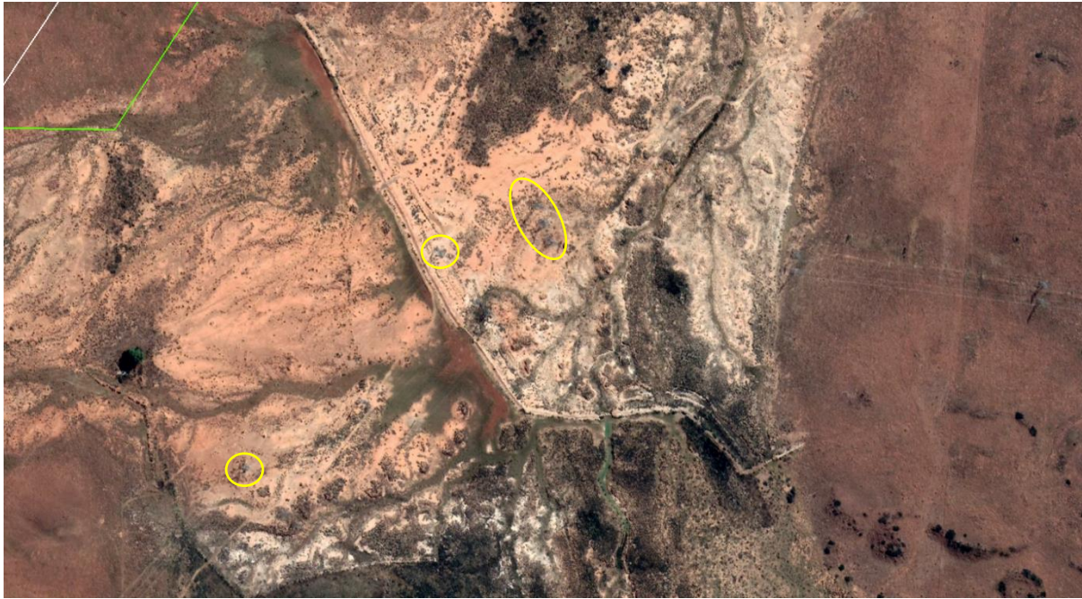
Figure 5-6 Illustration of existing in-stream weirs structures and powerline pylons (yellow circles) within the drainage features (Google Earth)
