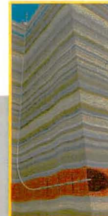
Hydraulic fracturing. A steel casing inside the well protects shallow fresh-water aquifers.
