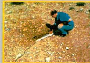
Placing magneto-tellurics sensors for geophysical data collection.
