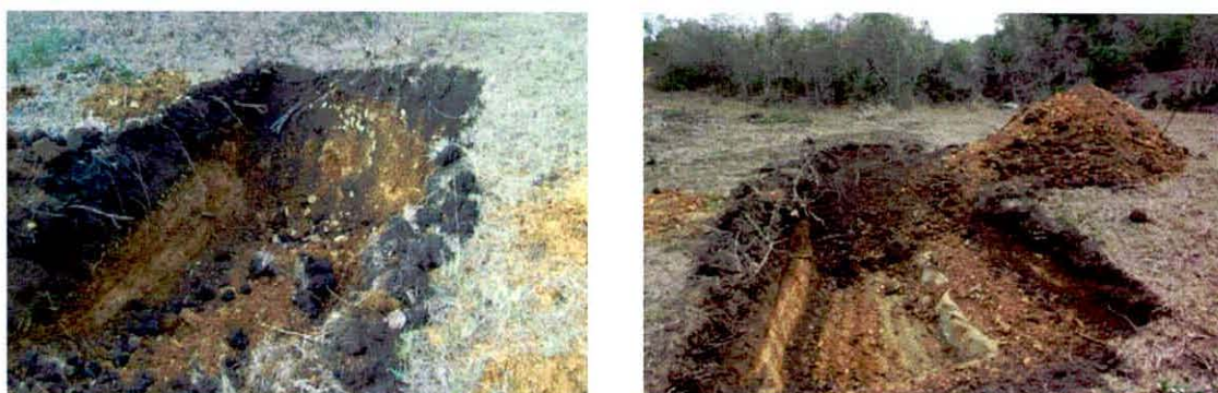
Figs. 5-6. Test pits 2 and 3 indicating shallow topsoil overlying weathered dolerite
