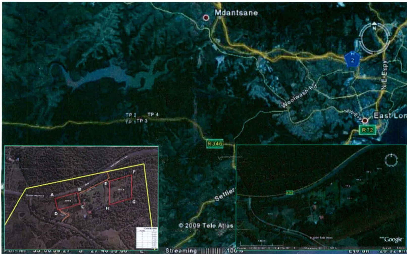
Map 2. Maps indicating areas and extent of proposed mining of weathered dolerite. Map A shows the borders for mining and access roads (map supplied by the consultants). Map B shows the test pits, GPS readings taken and extend of area surveyed
