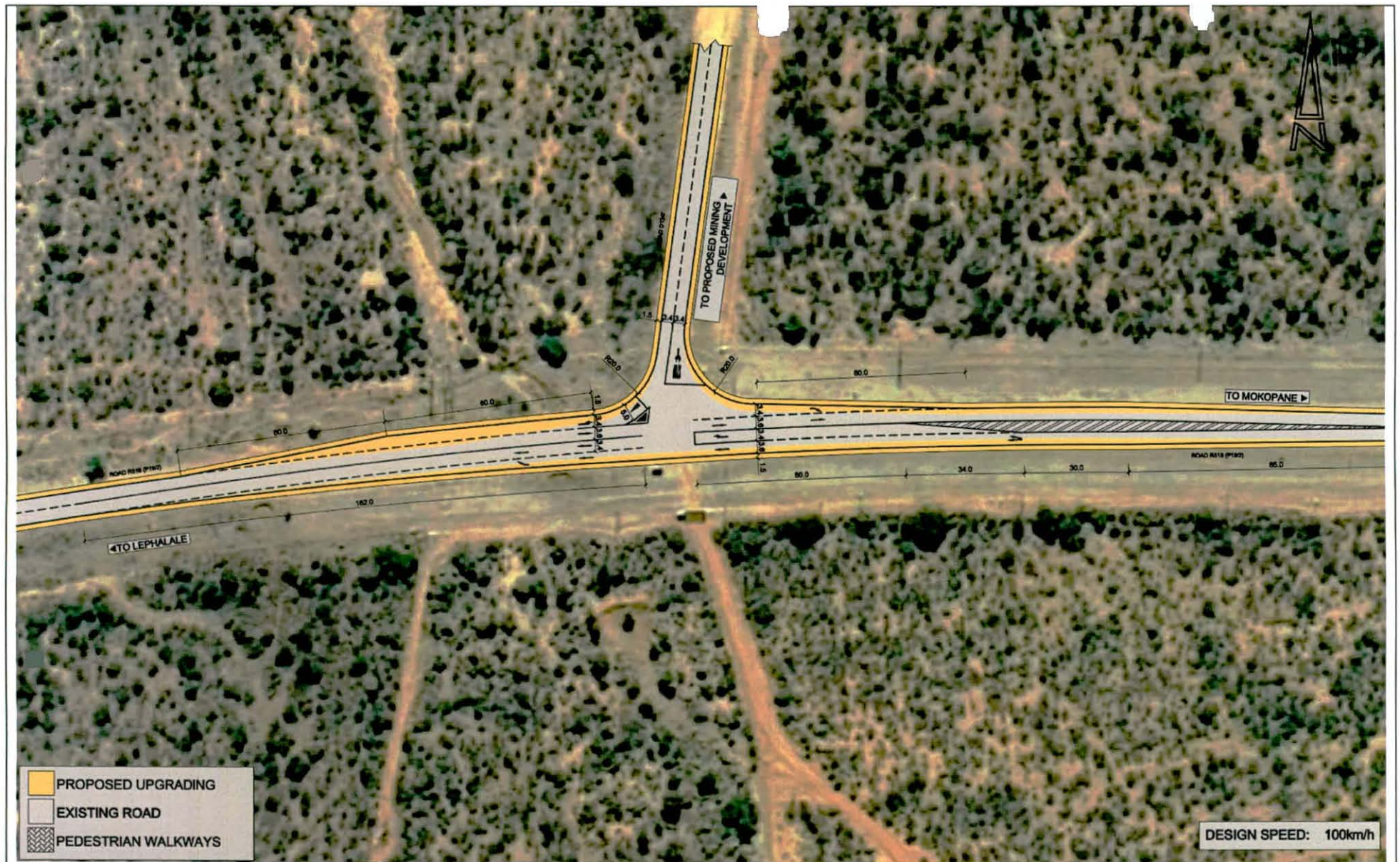
FIGURE 2.2: RECOMMENDED UPGRADING OF THE INTERSECTION OF ROADS R518 (P19/2) AND D1347 (POINT C)
