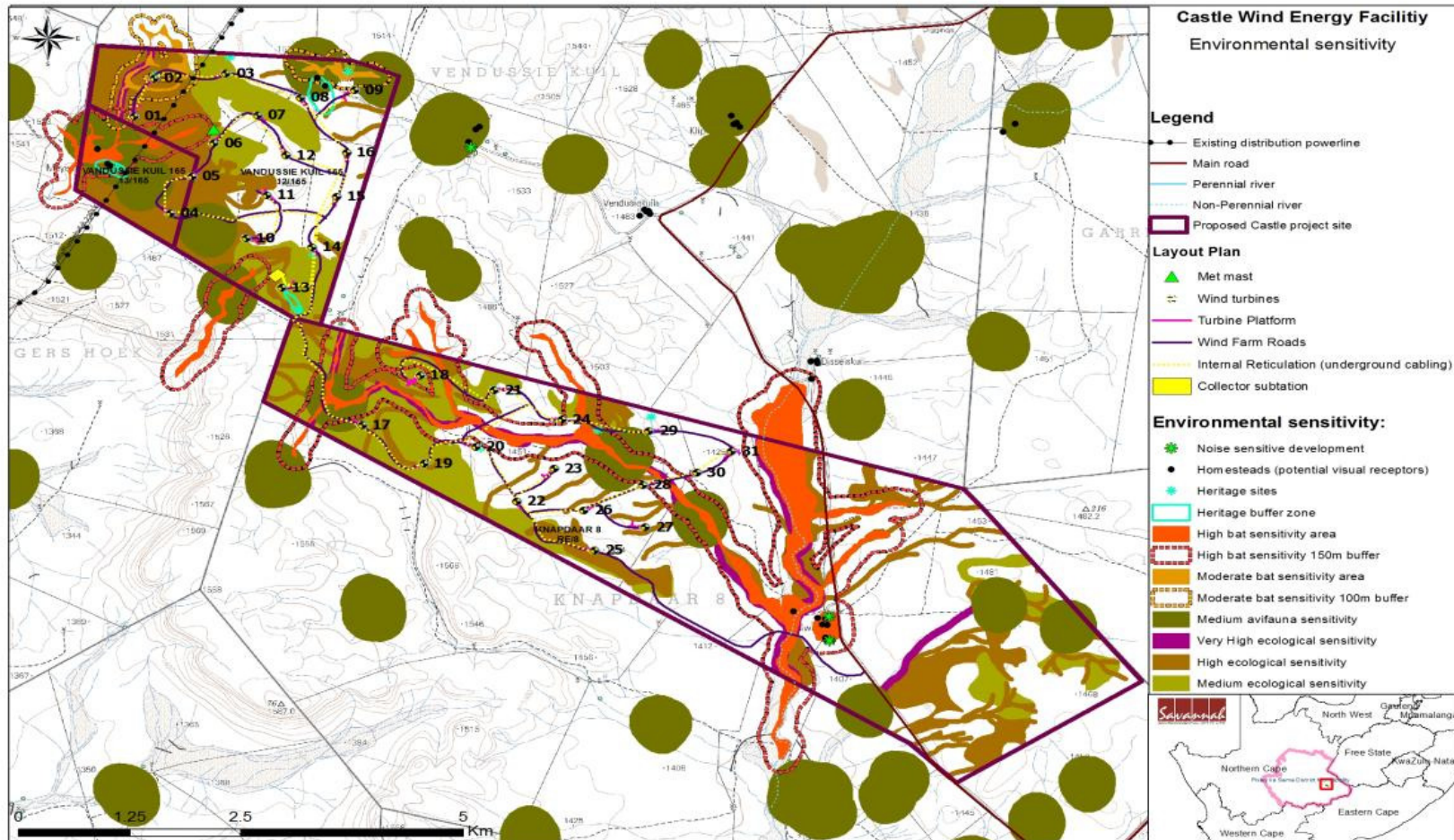
Figure 10.4: Environmental sensitivity map for the project study area illustrating sensitive areas in relation to the proposed development footprint for the Castle Wind Energy Facility ( Appendix P contains an A3 map)
