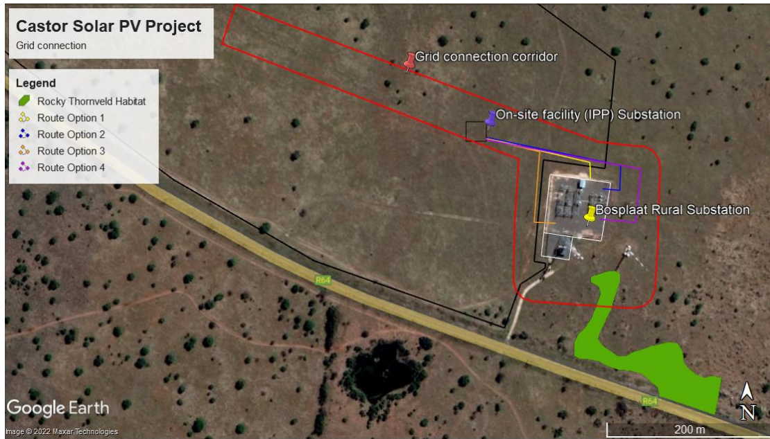
Figure 5.4: Final grid connection routes proposed for the Castor Solar PV Project within the assessed grid connection corridor
