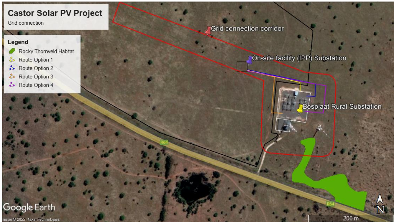
Figure 2.2: Final grid connection routes proposed for the Castor Solar PV Project within the assessed grid connection corridor
