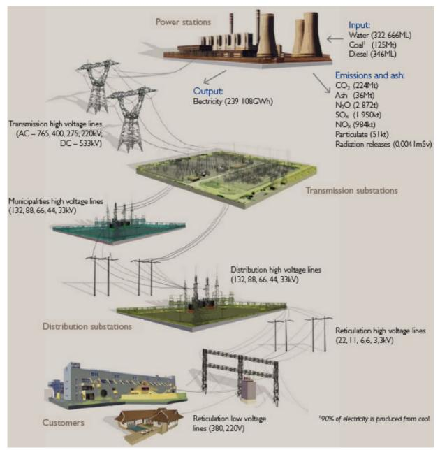
**Figure 3.1:** Simplified electrical transmission and distribution system (source: www.eskom.co.za)
