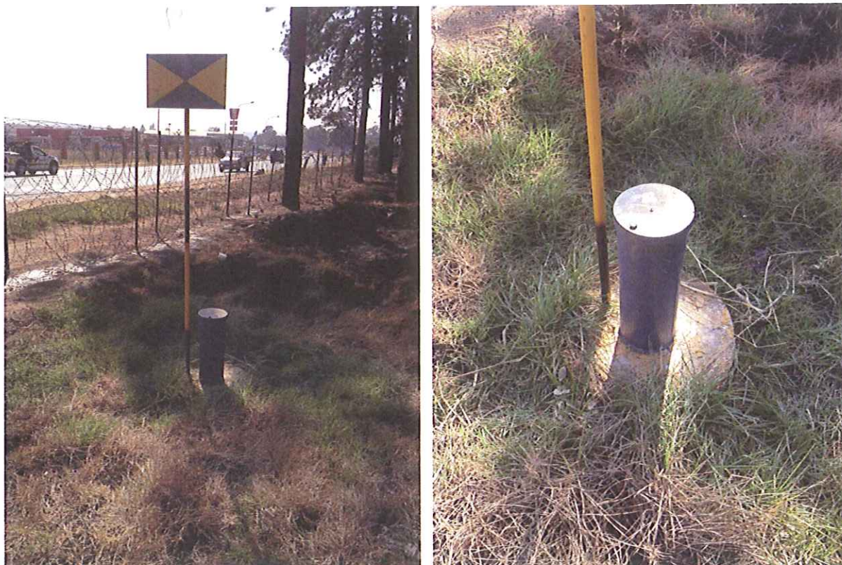
Plate 8-1: Example of a monitoring borehole
