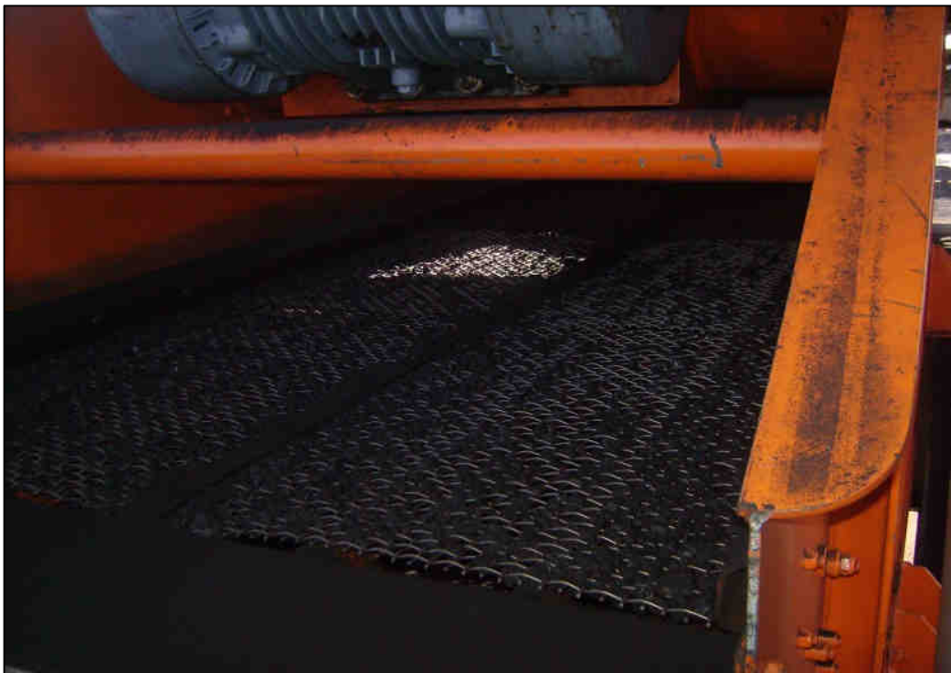
Plate 3.9: The vibrating screen – coal is passed over this screen to remove the unwanted fines less than 15 mm in size.
