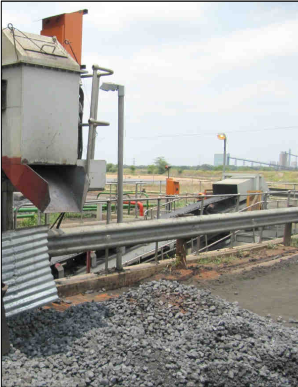
Plate 3.13: Quenched char leaving the retort.
