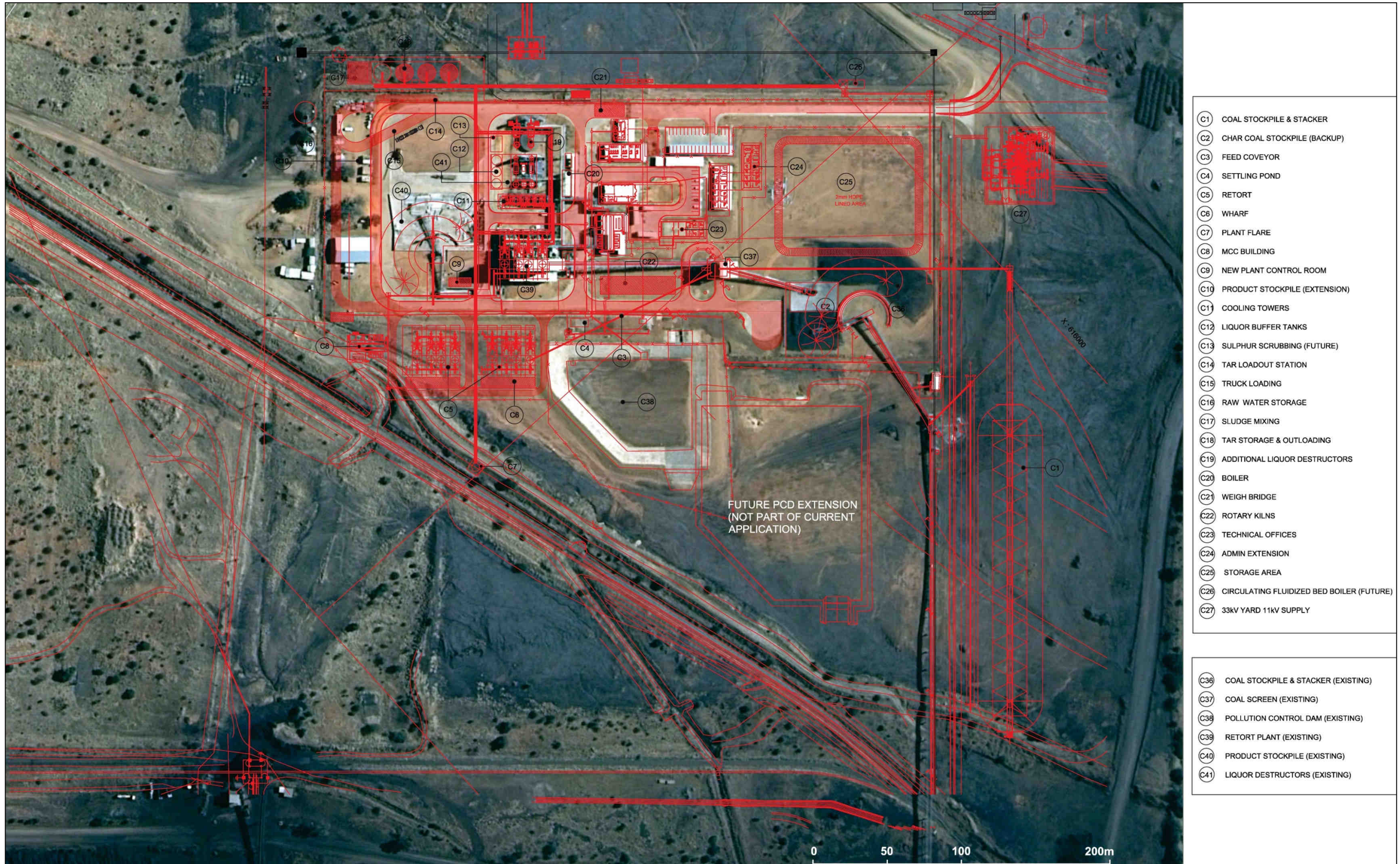
Figure 3.24: Layout of Char Manufacturing Plant Expansion showing an aerial view of the existing plant
