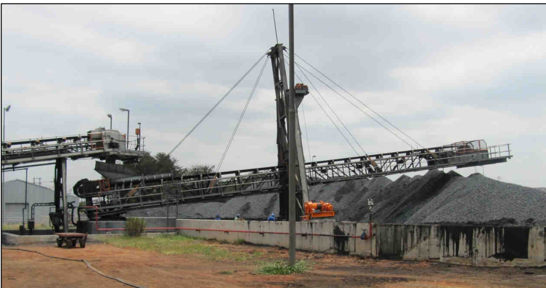
Plate 3.14: The product stacker stacking the char onto the product stockpile area.
