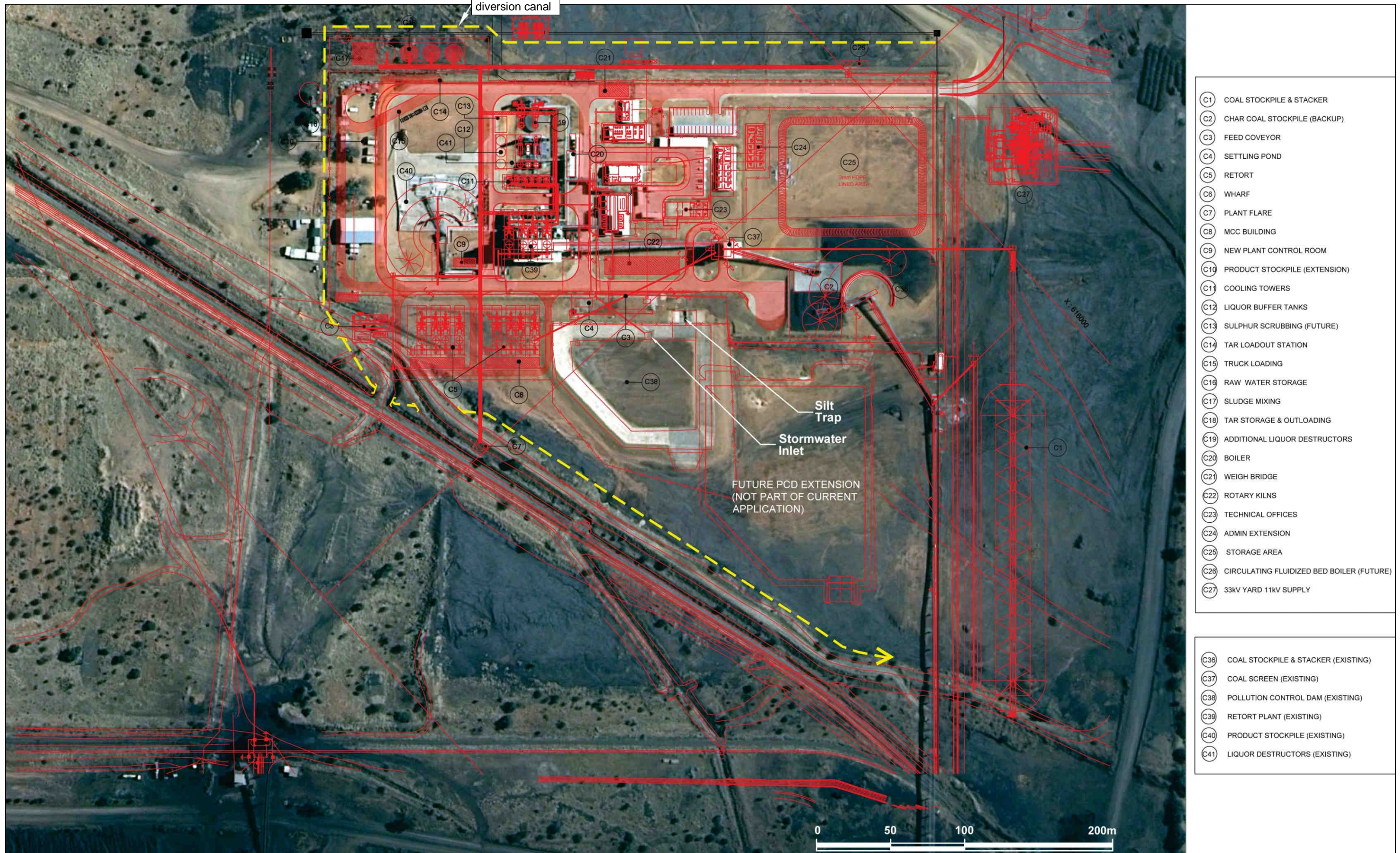
Figure 3.27: Layout of the stormwater management system for the Char Manufacturing Plant Expansion
