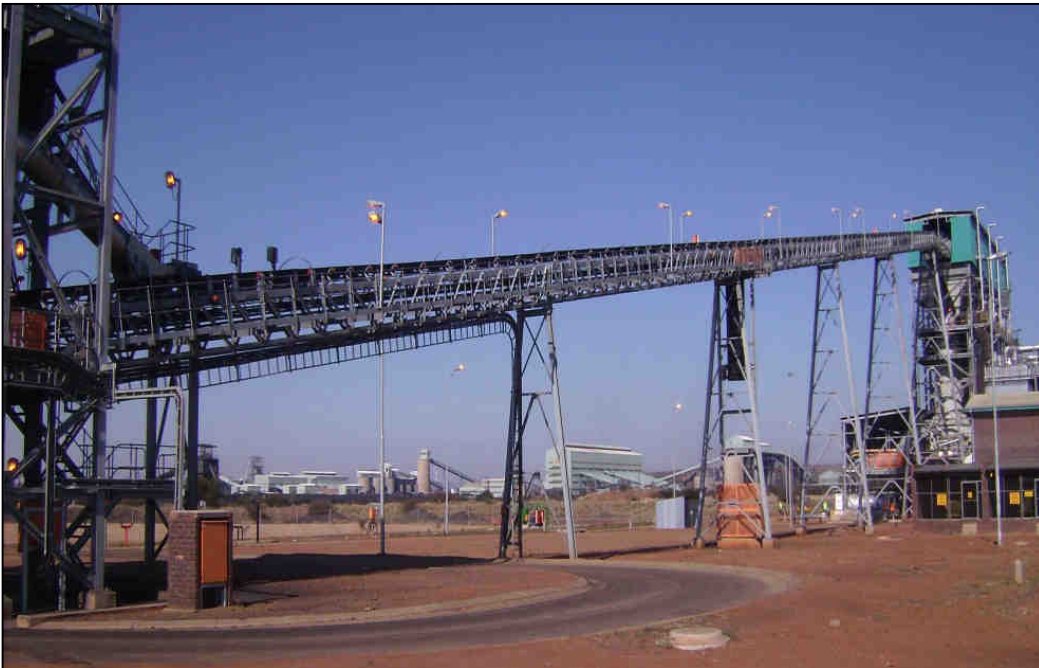
Plate 3.10: The screened coal is transported via conveyor belt to the retort feed bins located above the retorts.
