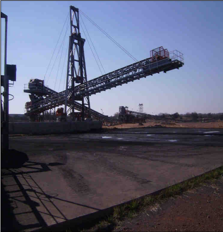
Plate 3.7: The coal from the mine is transported to the Char Manufacturing Plant via conveyor and is stockpiled on a concrete lined area.
