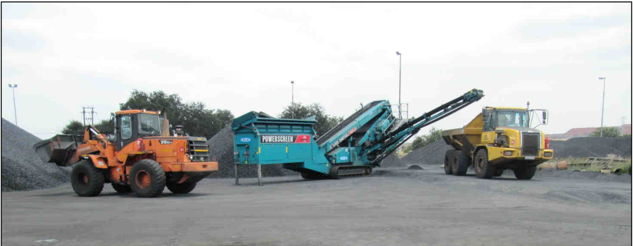
Plate 3.15: Char is stockpiled and separated (screened) into char fines and lumpy char.
