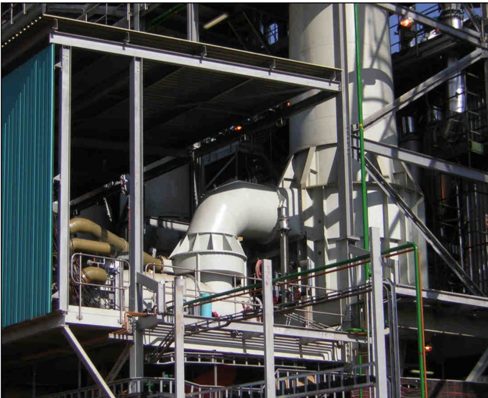
Plate 3.12: The retort in which the coal is heated.
