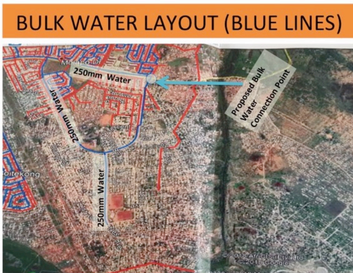
Figure 4: Existing Bulk Water Layout
