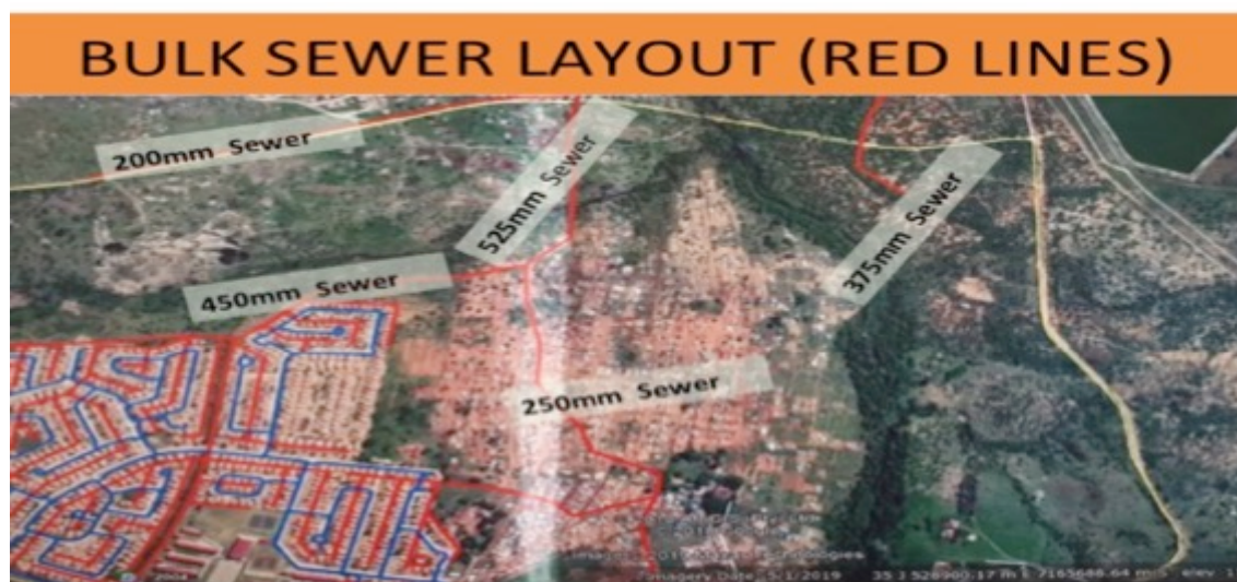
Figure 5: Existing Bulk Sewer Layout
