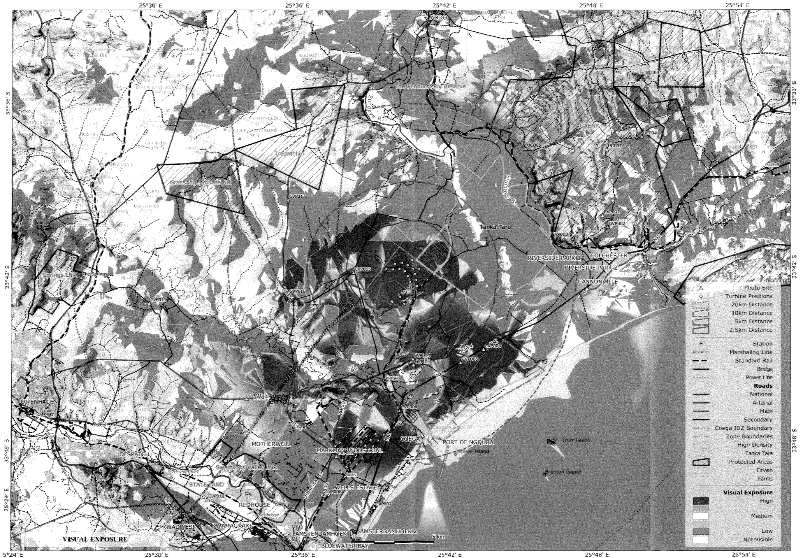
Figure 8.8-7 Visual exposure calculated from visibility and distance from nearest turbine. Sites visited for the photographic survey are also indicated.
