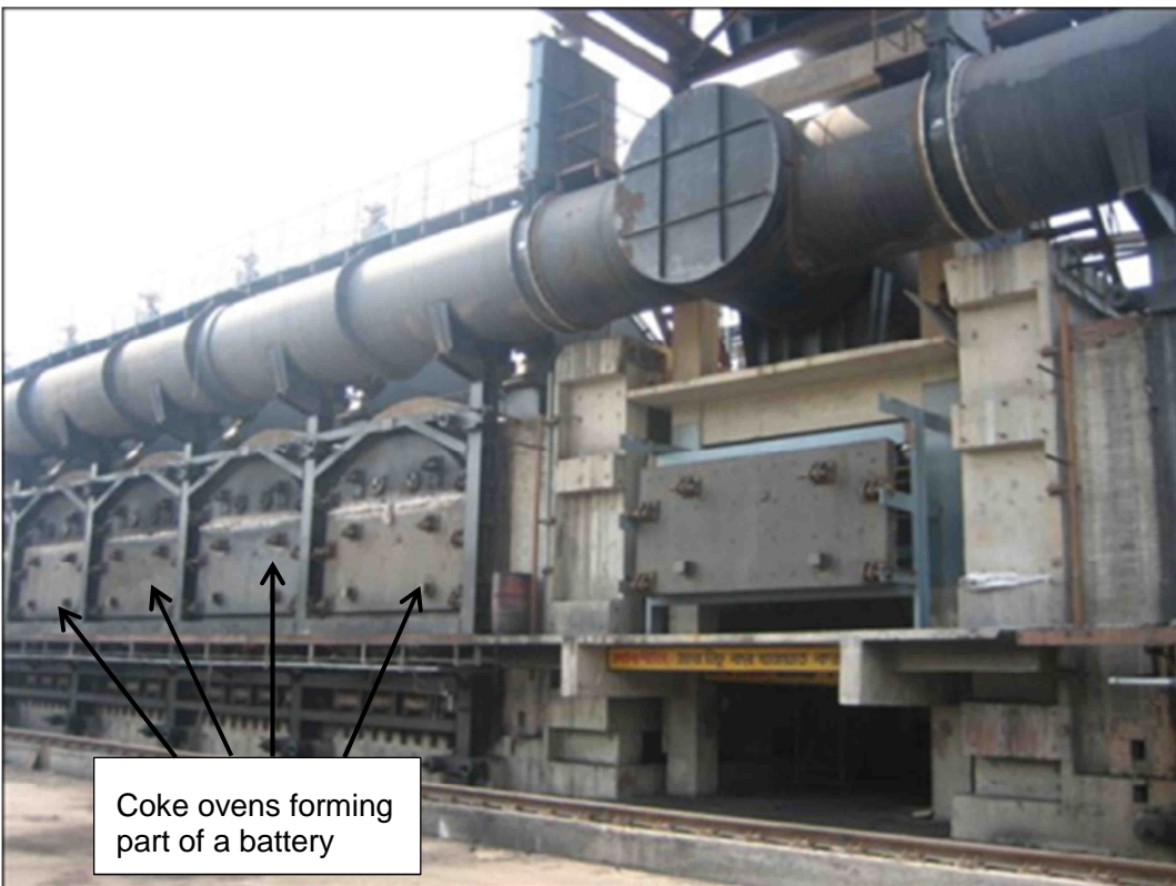
Figure 2.4: Part of a coke oven battery (similar to proposed Market Coke Plant).
