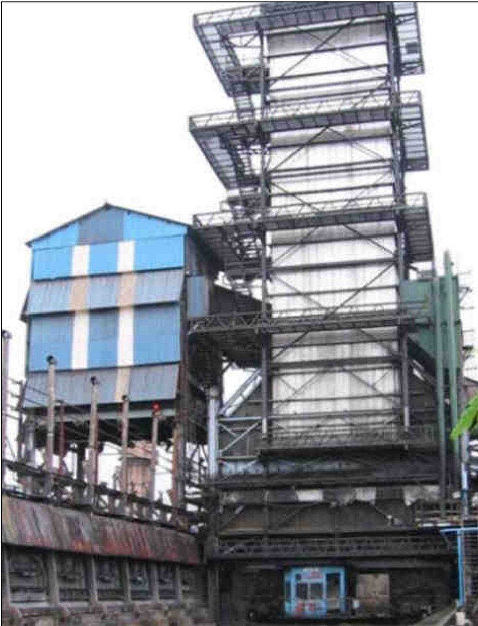
Figure 2.9: Typical quenching tower with quenching car underneath the tower (similar to proposed Market Coke Plant) (Courtesy Sesa Goa Ltd).
