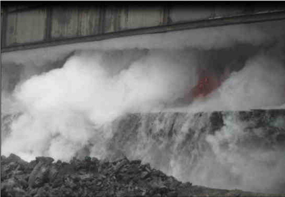
Figure 2.10: Coke cake undergoing quenching (Courtesy Sinosteel).
