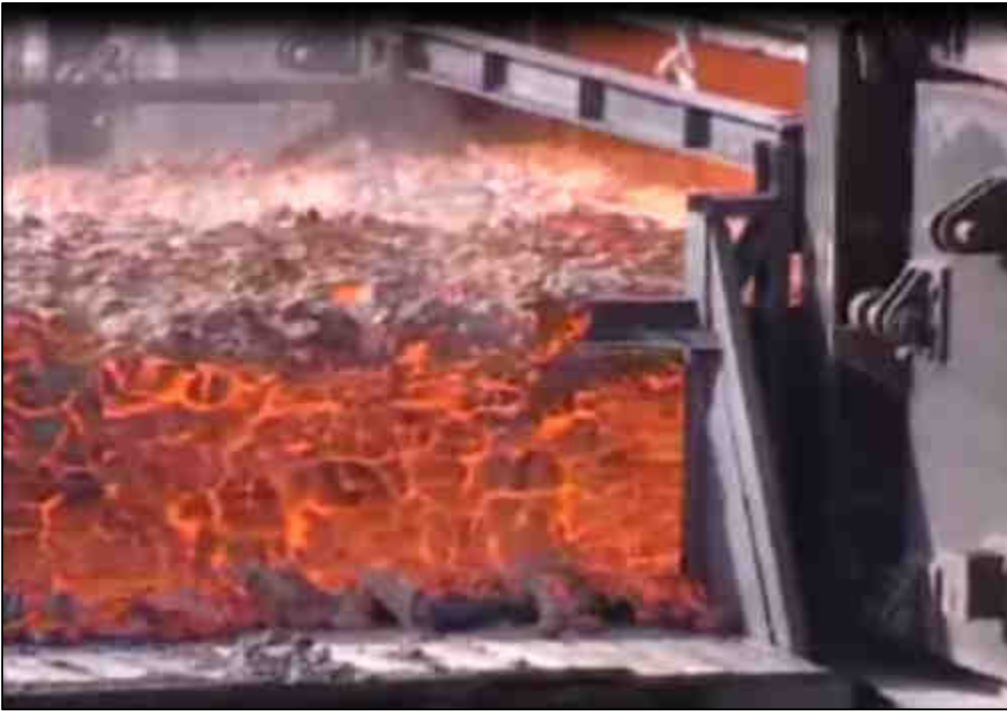
Figure 2.6: A coke cake which has been heated and is being pushed out of the coke oven (Courtesy Sinosteel).
