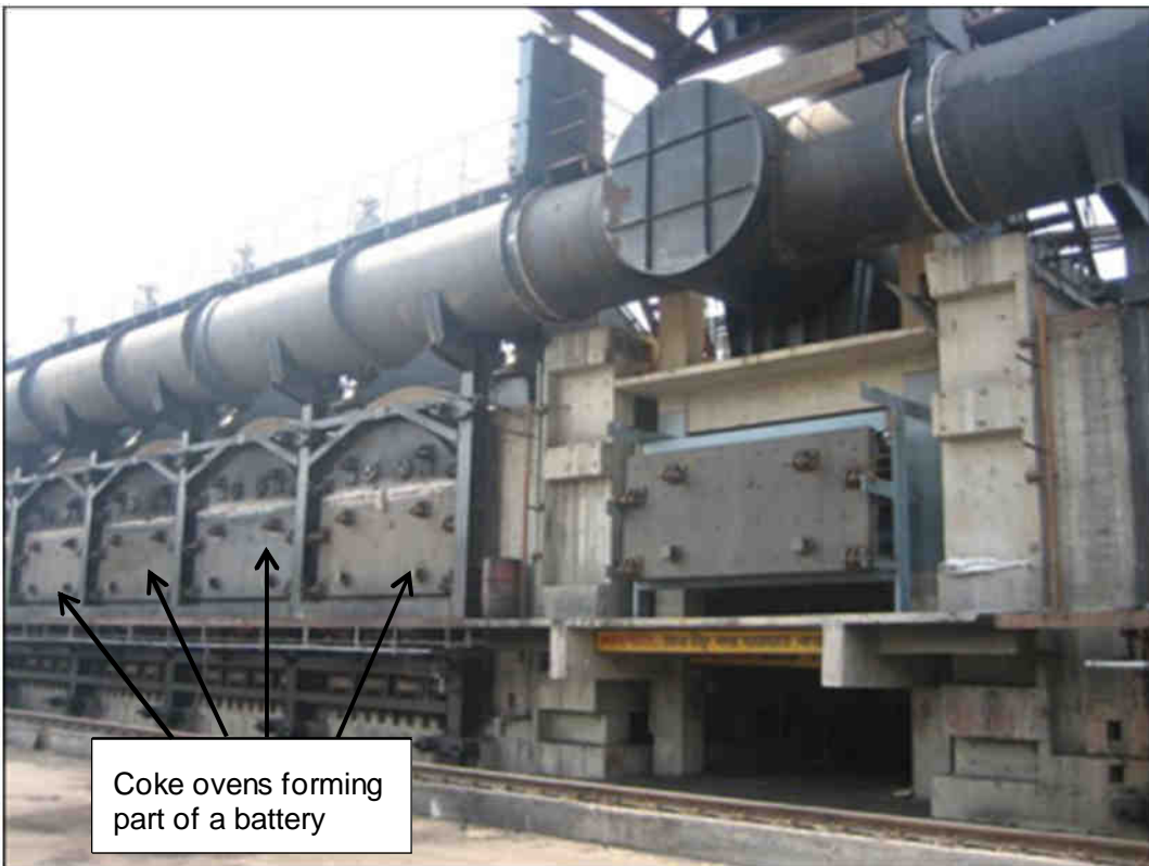
Figure 3.7: Part of a coke oven battery (similar to proposed Market Coke Plant).
