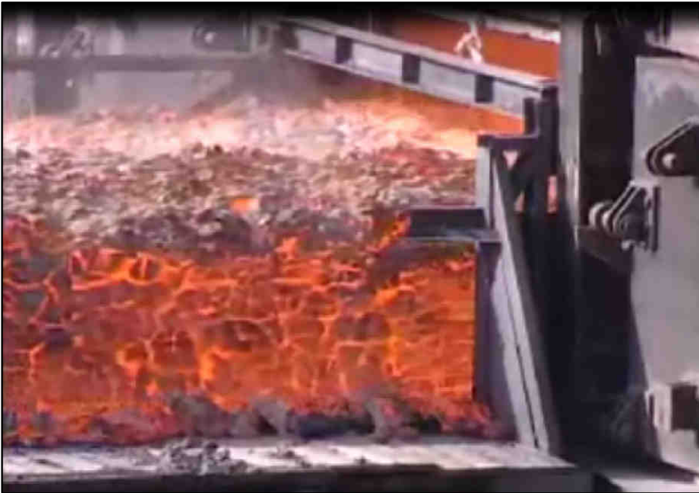
Figure 3.9: A coke cake which has been heated and is being pushed out of the coke oven (Courtesy Sinosteel).
