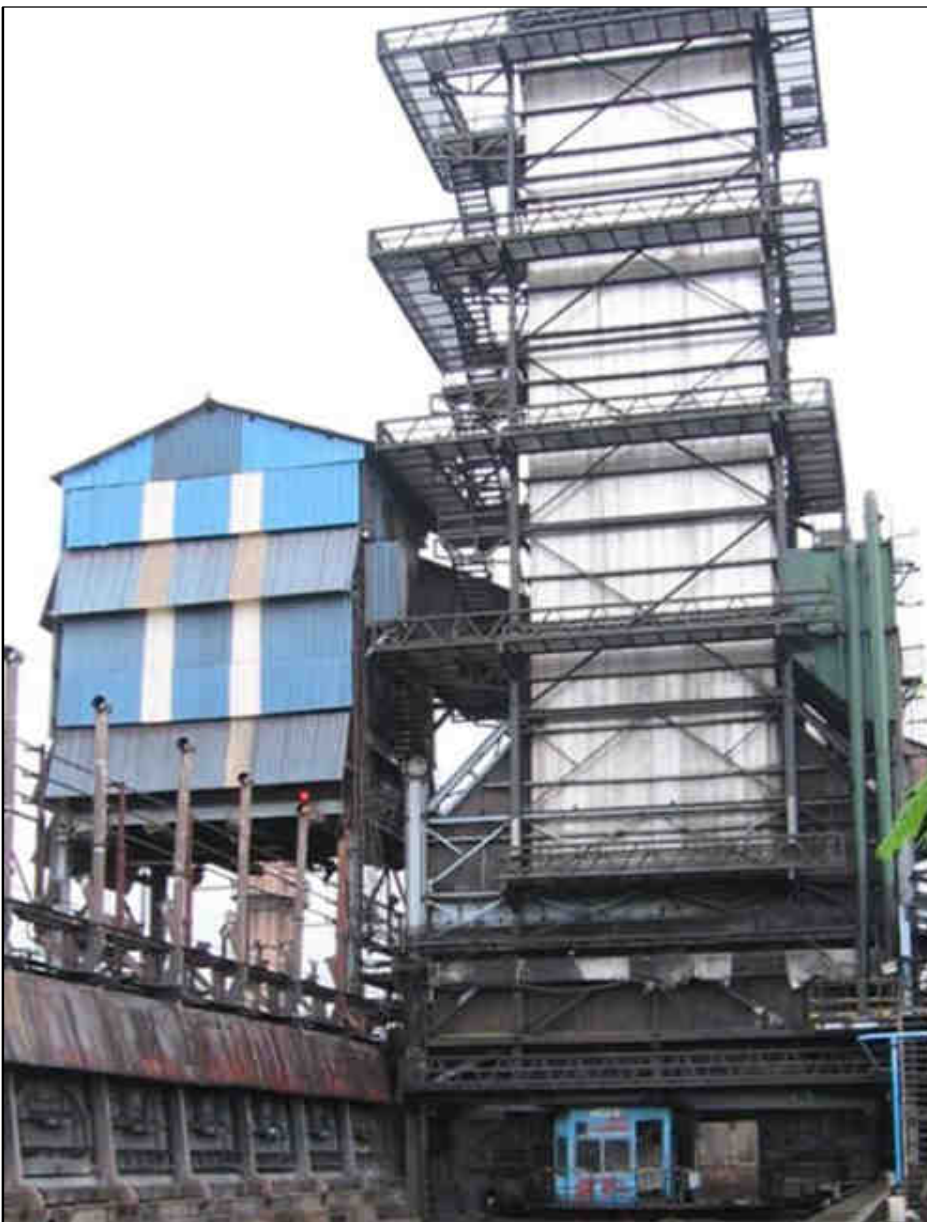
Figure 3.12: Typical quenching tower with quenching car underneath the tower (similar to proposed Market Coke Plant) (Courtesy Sesa Goa Ltd).
