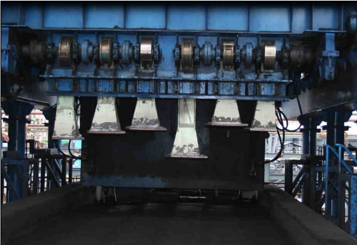
Figure 3.6: Coal cake being compressed by stamping machine (Courtesy Sinosteel)
