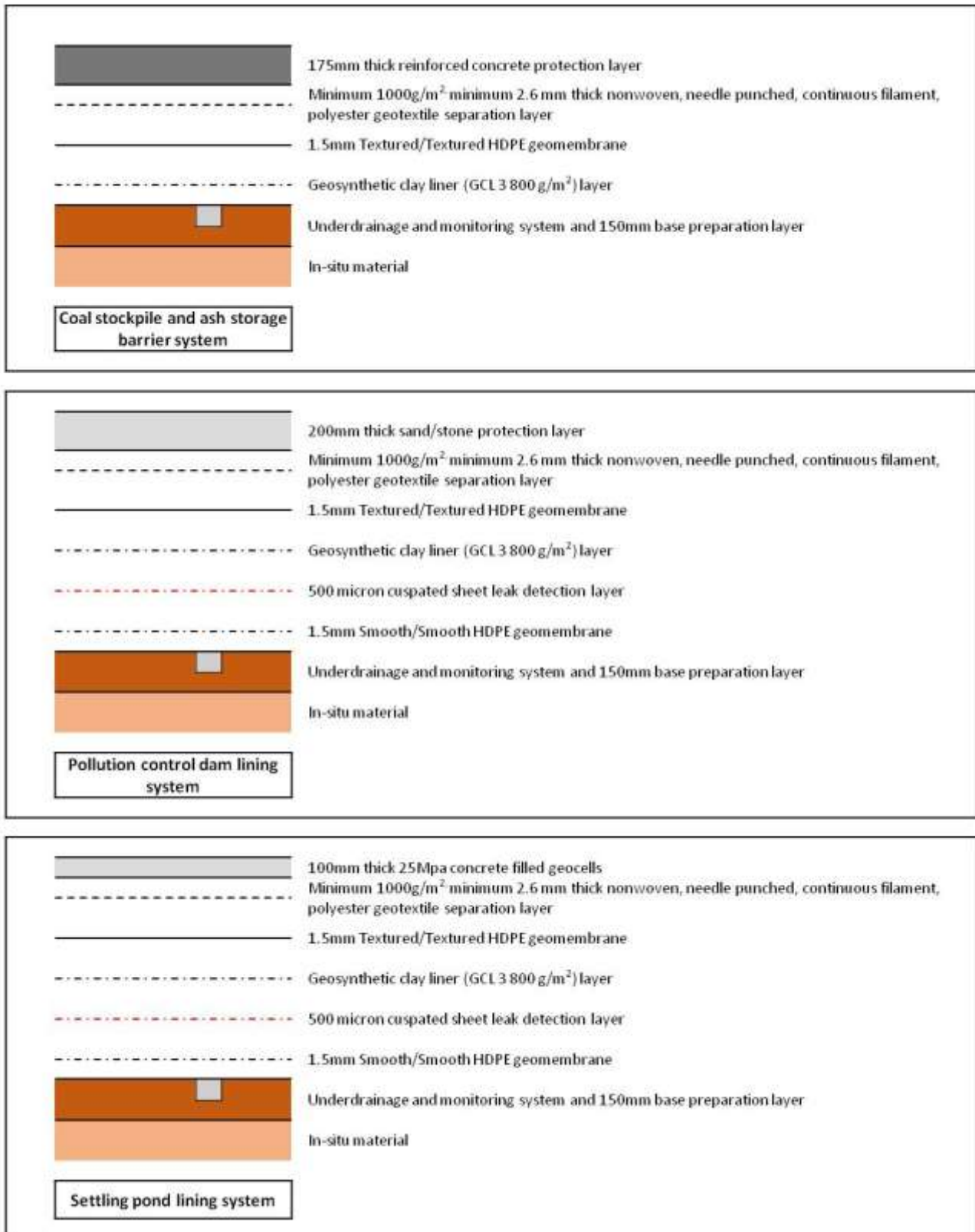
Figure 2-12: Landfill barrier design
