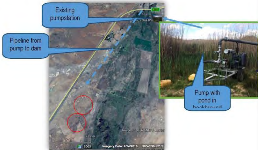
Figure 3: Existing pumpstation and line to pivots
