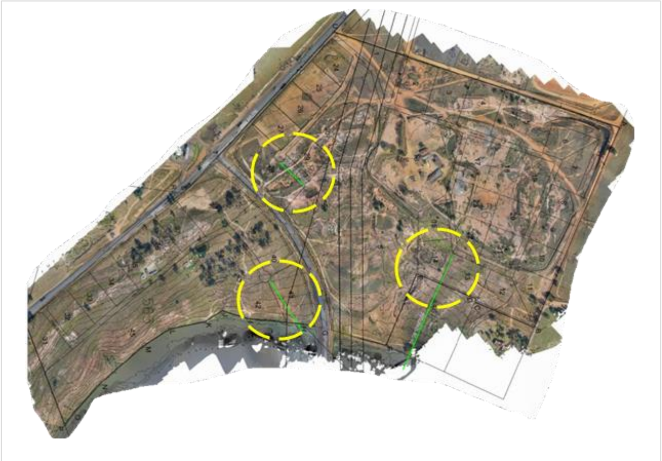
Figure 5: Flow of stormwater on the property
