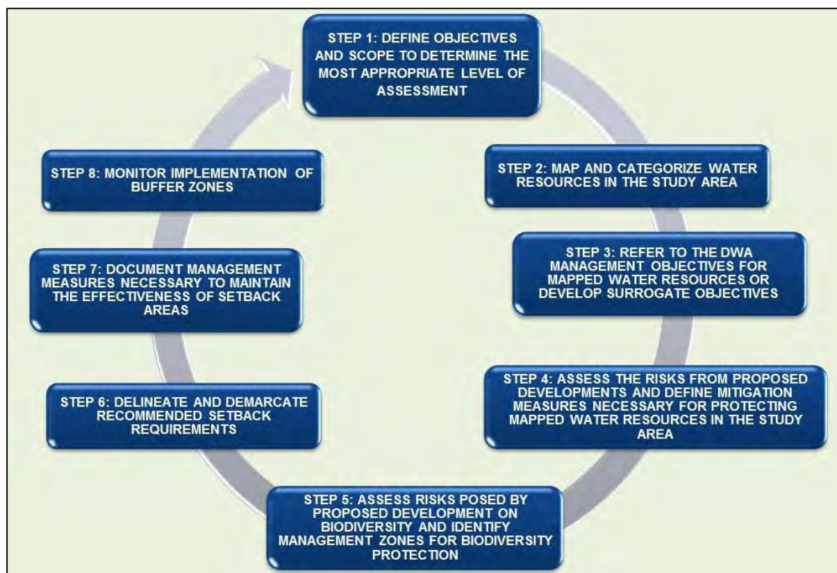
Figure 4-2: The assessment for the determination of the appropriate buffer zone follows this procedure
