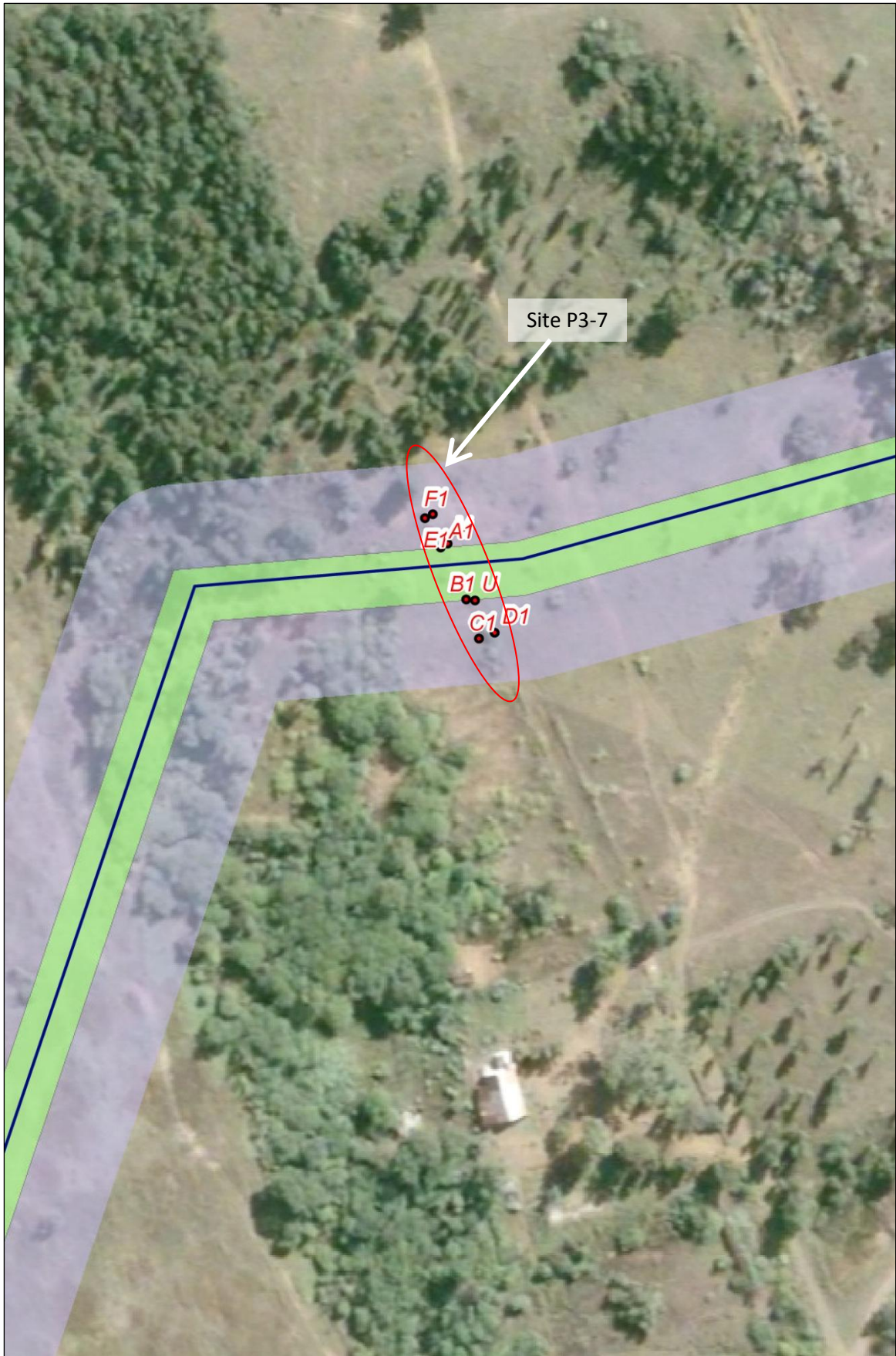
Figure 3 – Rand Water plan depicting the proposed pipeline route (depicted as a dark blue line) in relation to Site P3-7.
