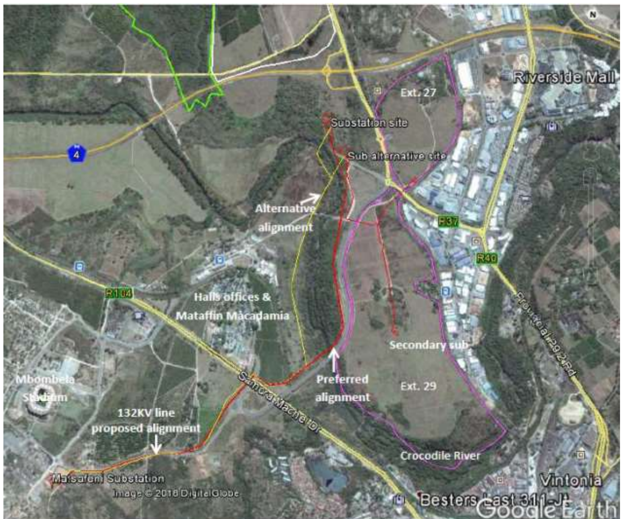
Figure 1: Powerline and substation alternative layout
