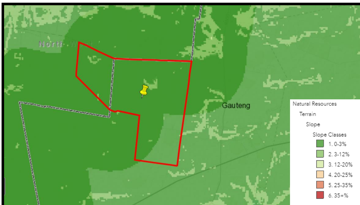
Figure 6: The slope class of the study area consists of the lowest slope class: 0-3% and 3-12%. The terrain is therefore considered relatively flat and suitable for a solar PV development.
