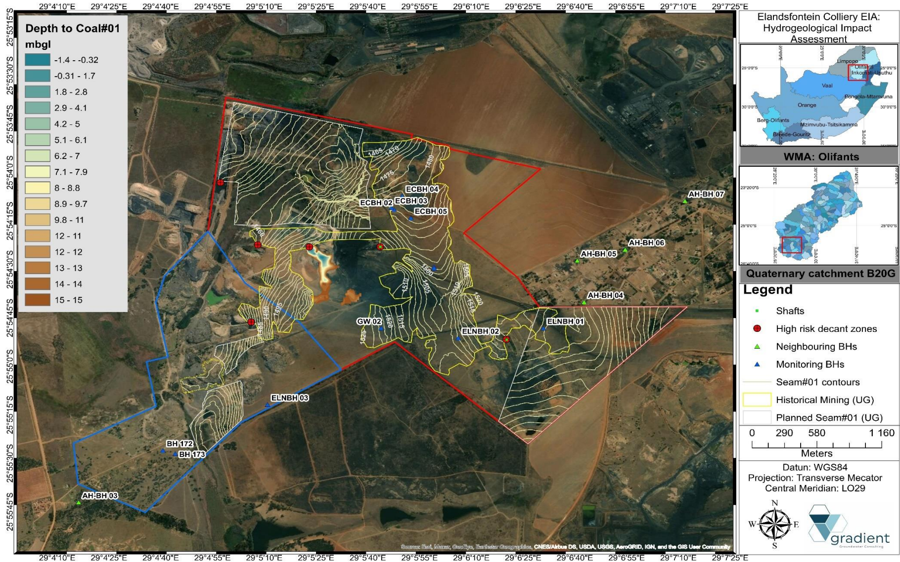
Figure 12-26 Scenario 03b: Potential high-risk decant zone for the underground mine void.
