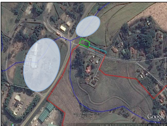
Figure 3: Wetland areas shaded in blue with the pipeline route illustrated in red. The proposed pump station is shown in green.
