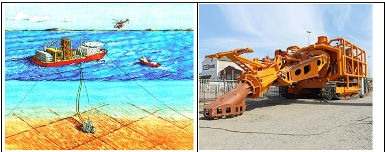
FIGURE 3-3: SCHEMATIC DIAGRAM SHOWING OPERATION OF A SEABED CRAWLER AND PHOTOGRAPH OF SEABED CRAWLER.
