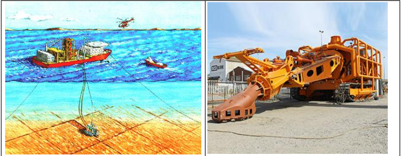
Figure 4-4: Schematic diagram showing operation of a seabed crawler and photograph of seabed crawler
