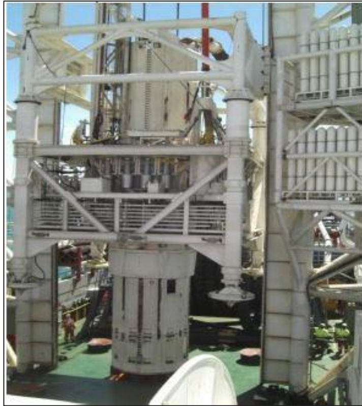
Figure 3-6: Illustrative example of drill bit operated from a drill frame structure located onboard a vessel of opportunity.
