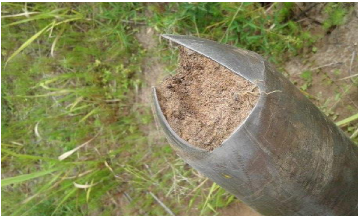
Photo 6: An example of the light brown sandy soils extracted from a drainage line within the study area, note the absence of wetland indicators.
