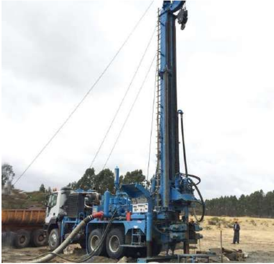
Figure 6: Typical example of air flush drilling machine with the drill bits.
