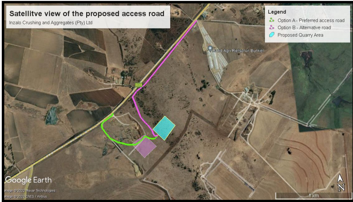
Figure 6: Satellite view showing the preferred access road (green line) and the alternative road (pink line) to the proposed mining area site alternative 1 as well as the site alternative 2 (pink polygon)
