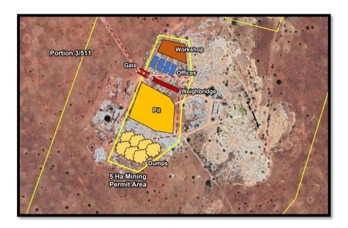
Figure 2: Site Layout Plan of the proposed Quarry.
