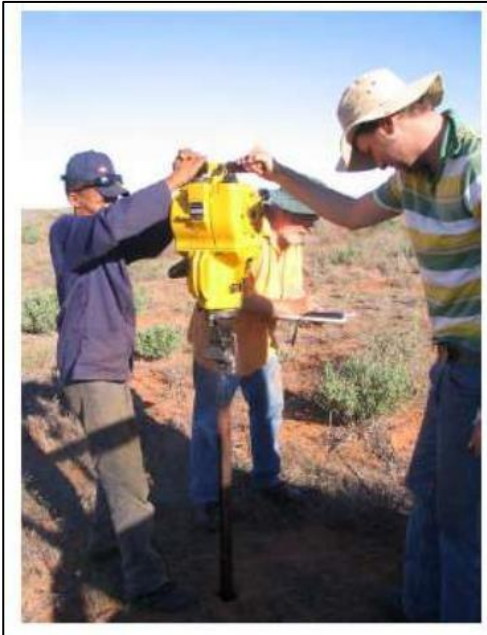
Figure 4 – An example of a hand held engine driven auger drill
