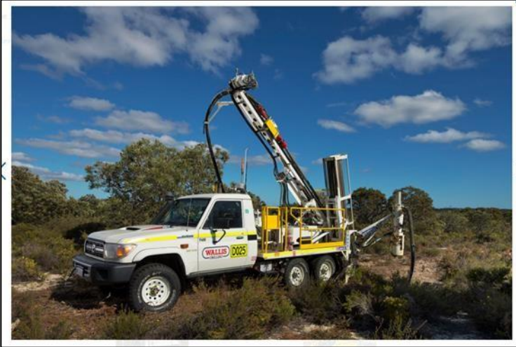
Figure 5 – An example of an Air-core drill mounted on the back of a Land Cruiser.
